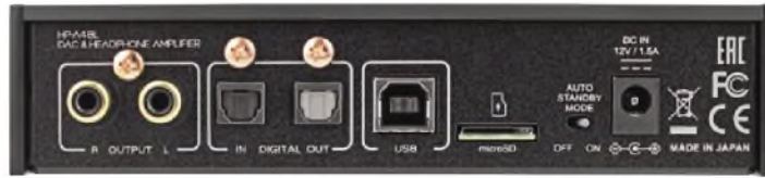
Rear phono audio outputs allow connection to a hi-fi system and there's also a digital out. The microSD slot cannot be used for anything other than firmware updates.
