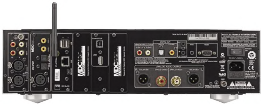
The well-stocked rear of the NAD Master Series M12 pre-amplifier. Note the fitting of the optional MDC panel (with aerial) which allows wireless communication with the Bluesound Vault 2.
