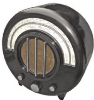
Ekco AD65 AC/DC superhet radio, introduced 1934, a classic built of Bakelite.
