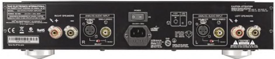
The NAD Master Series M22 power amplifier has both balanced and unbalanced audio inputs as well as sturdy gold-plated 'speaker binding posts'.
