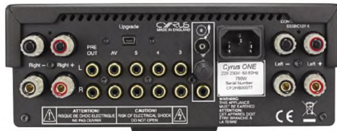
A crowded rear panel contains analogue line inputs, plus a phono input for LP. There is a pre-amp output too, and Bluetooth offers digital connection.
