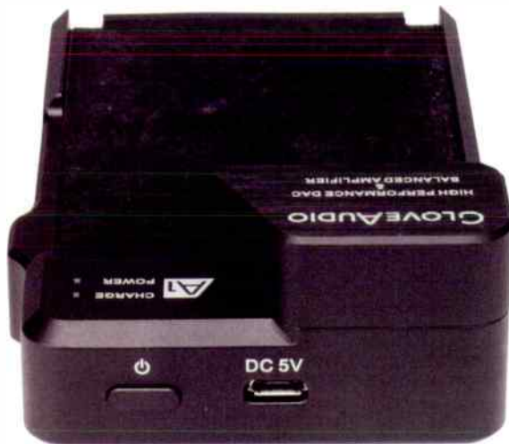
At top lies a power on/off button and micro-USB socket, to charge the internal battery.
