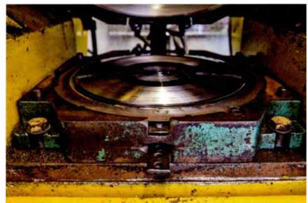
The pressing machine is sturdy, to resist high pressure needed to form the heated vinyl against the stampers.
