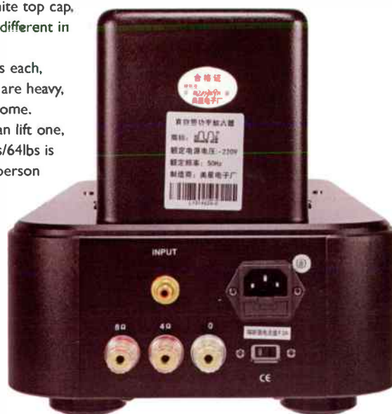
The rear carries a single phono socket input and an 8 Ohm output, with 4 Ohm tap, that uses strong gold plated binding posts.
