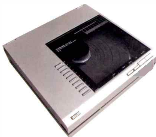
Technics SL15 Direct Drive turntable, with short, parallel tracking arm in the lid holding a T4P mount plug-in cartridge. Almost as automated as a CD player.
