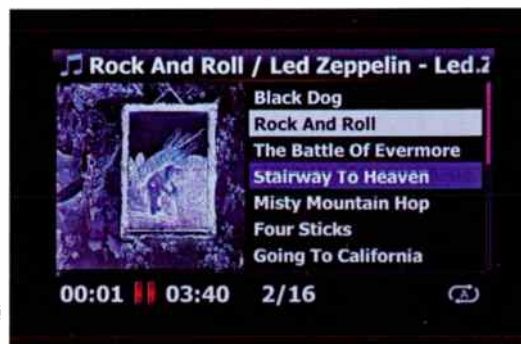
The TFT front panel display can show album artwork plus a variety of information on the track being played.
