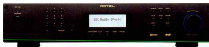
"Rotel RT-12 tuner unfortunately has no digital outputs" says Jim Thorpe. "A budget ADC is needed".
