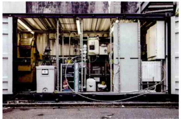
Marclay's vinyl is created using the world's first mobile vinyl pressing plant...situated in a shipping container.
