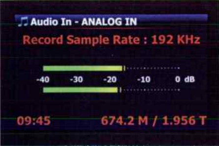
An analogue input allows for the recording of LPs to the hard disk at 192kHz.
