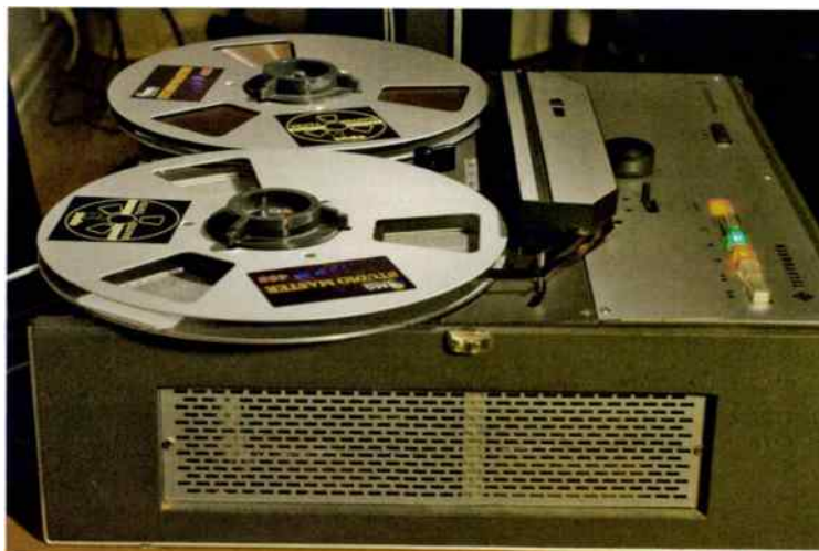
The Telefunken Magnetophone M28C that is used to make the tape master copy for all Opus 3 analogue recordings.
