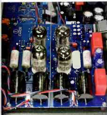
The pair of Sovtek 12AX7LPS and the two 6922 valves act as the amplification for the analogue output stage.
