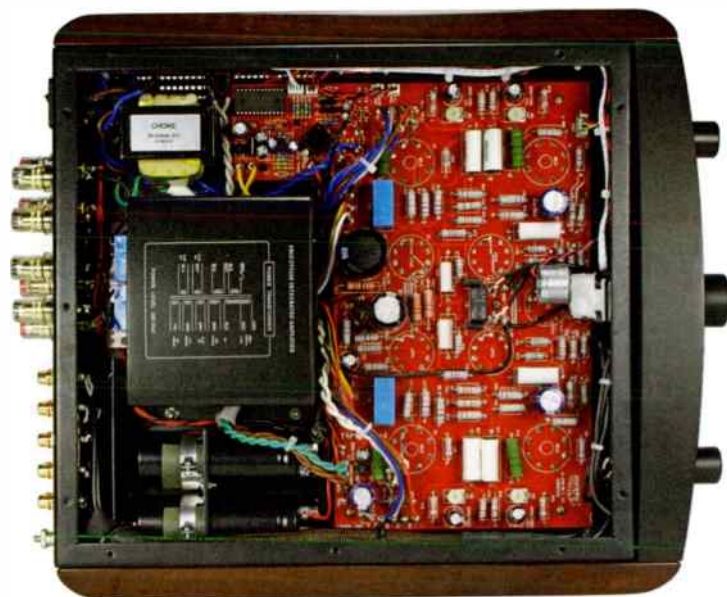
Neatly laid-out internal circuit board, mains transformer and black PSU capacitors; Alps motorised volume control at right.
