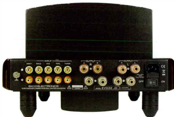
The power switch is placed under the mains plug – an awkward positioning. Input sockets are high quality and two pairs of loudspeaker outputs can be switched.
