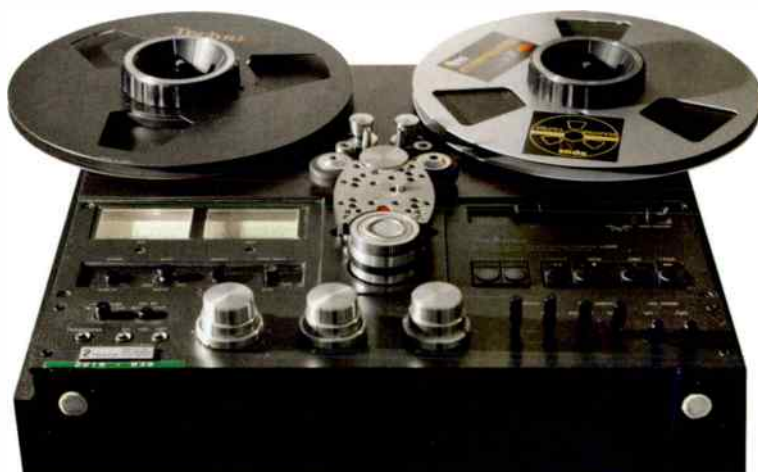
The Technics RS1500U used to playback the mastertape when recording copies, such as the tape used in this review. It is modified to have IEC/CCIR equalisation, rather than the NAB equalisation of the standard machine.
