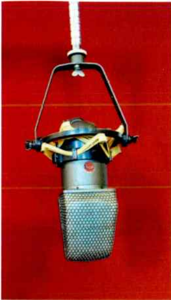
An original (1959) RCA KU3A ribbon microphone. It's rarity falls into the hen's teeth category.
