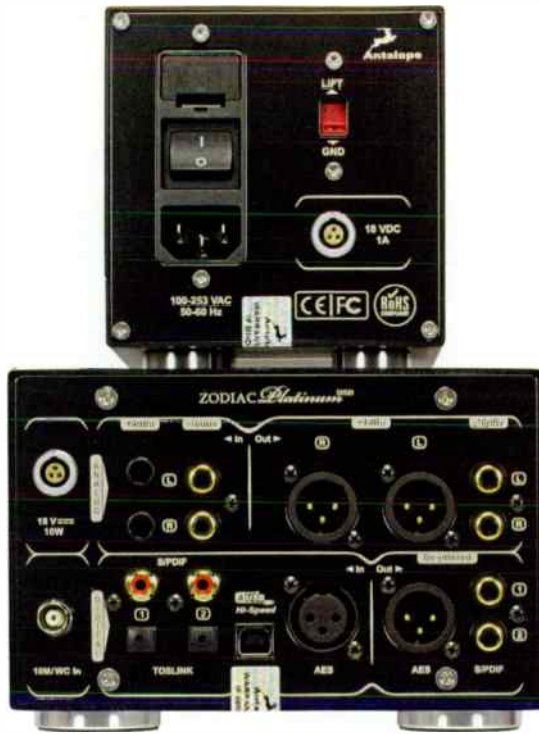
USB, plus AES/EBU, optical and and electrical S/PDIF inputs, plus analogue inputs and outputs in balanced (XLR) and unbalanced form. There's clock input too.
