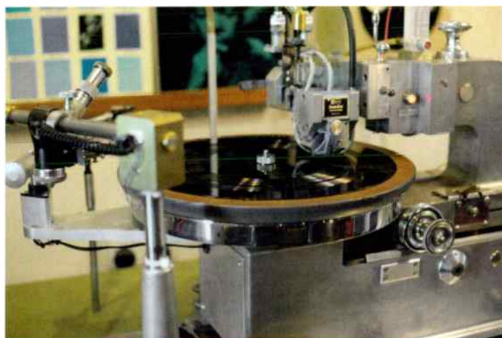
A Scully lathe with Westrex cutting heads and amps – truly analogue.
