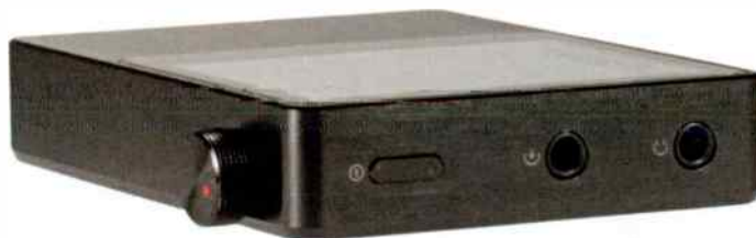
The top face carries and on/off button (left, optical digital input and, at right, headphone output that incorporates an optical S/PDIF digital output.
