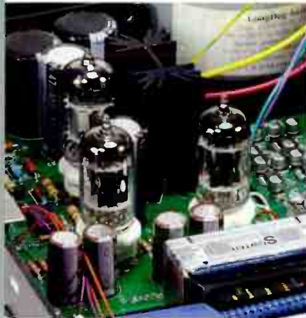
Two 5687 triodes and an EF86 RF pentode give the Longdog DAC a distinctive, punchy sound.
