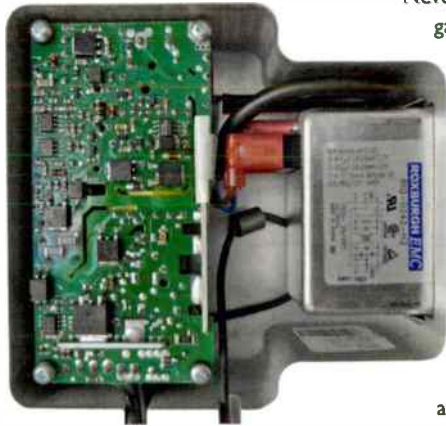
The power supply section is built into a separate enclosure within the machined case to minimise interference.
