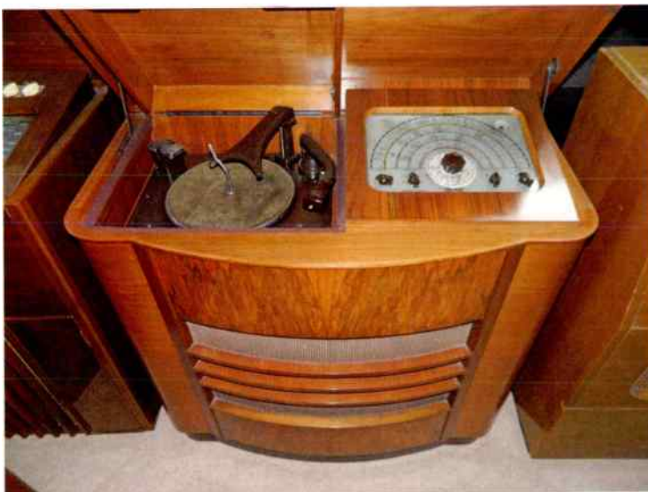
The radiogram – an all-in-one music playing system as the world once knew it, complete with wood and Tygan finish. The record deck invariably had a crystal cartridge. Better examples now fetch big prices, all the same.
