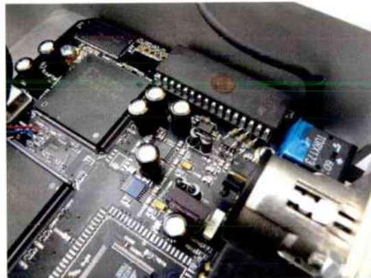
An EPROM chip (the device with the round sticker) stores the DAC 64's innovative firmware. It's 'pluggable' for upgrade purposes.
