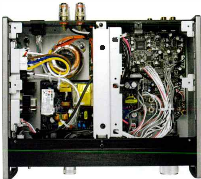
Here's a view of the AI-501DA's innards. The small toroidal transformer forms part of the small-signal stage's linear power supply. Beneath this, a switch-mode supply looks after the Abletec Class-D power amp.
