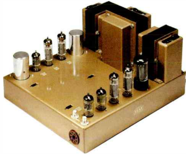
The Leak Stereo 20 amplifier, owned by Stuart Dunbar-Dempsey – a beautiful sound, but it has limited power and the output transformers saturate quickly with subsonics from LP.
