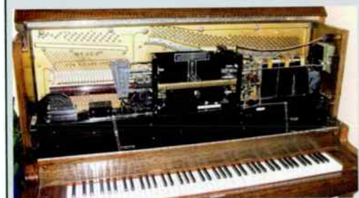
The lower half of the Aeolian mechanism in a Weber Duo-Art machine. (Image courtesy of http://justpianos.com.au )
