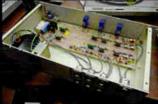
This electronic-crossover, containing a series of filters based around TL072 op-amps to split a line-level source into high, mid and low bands, was going for for a tenner. Great for active-speaker experimentation!
