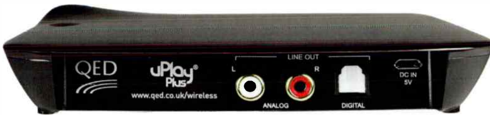
The rear panel carries analogue outputs, and an optical digital S/PDIF output. The QED has been designed for connection into a typical stereo amplifier, a DAC or a 'digital' amplifier with an on-board DAC.
