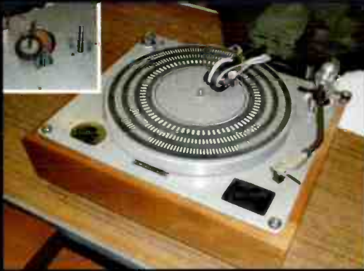
With a Lenco L75-S tonearm, this mint Sugden Connoisseur was selling for £300. A late-'50s Garrard 301 competitor, it coupled idler-drive with a tapered motor-shaft to achieve continuously-variable speed.
