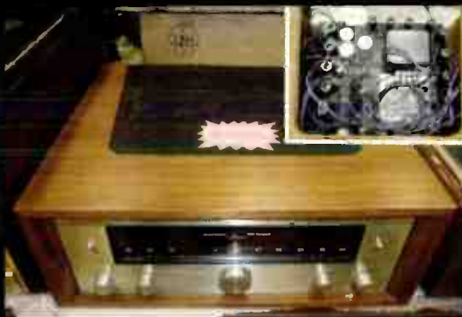
In 1963 Marantz apparently lost money on every 10B tuner, a beautifully-engineered FM-only classic with onboard oscilloscope. A front-panel scratch (and FM's numbered-days) makes this sample's £2000 asking price optimistic.
