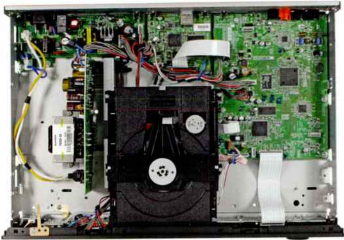
The CD tray and disc clamp dominate the internal space, showing just how bulky optical disc mechanisms really are. To the right lie numerous digital signal processing chips, and to the left the power supply.
