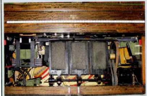
The top part of a Weber Duo-Art Player Piano showing the Aeolian mechanism. The paper roll fits into the black housing in the centre and engages with the lower roller. (Image courtesy of http://justpianos.com.au )
