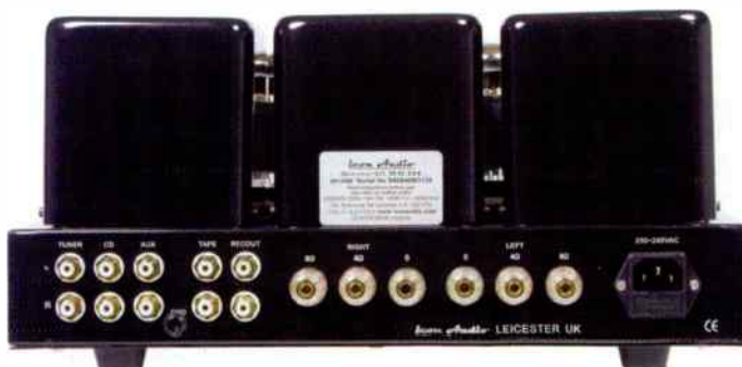
The 4 Ohm output of a valve amplifier will easily drive 3 Ohm loudspeakers.
