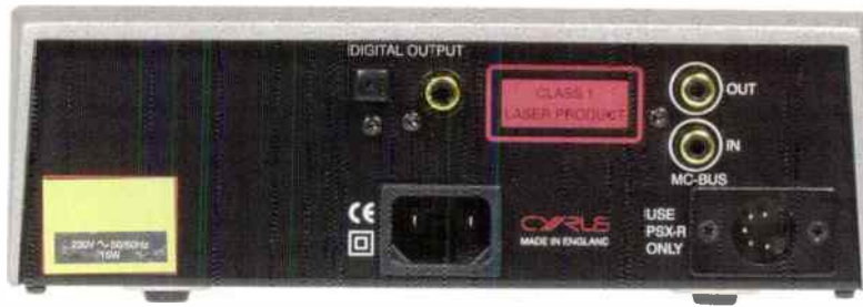
Only basic optical and coaxial digital outputs on the back; bottom right is the socket for the optional PSX-R external power supply.
