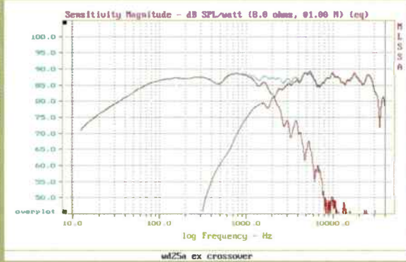
Figure 3. Measured results from WD25A EX showing acoustic crossover and response on treble unit axis.
