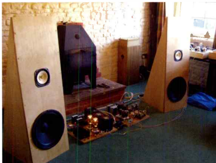
Typical enthusiasts free space placement of open baffle speakers (picture courtesy World Designs Forum).
