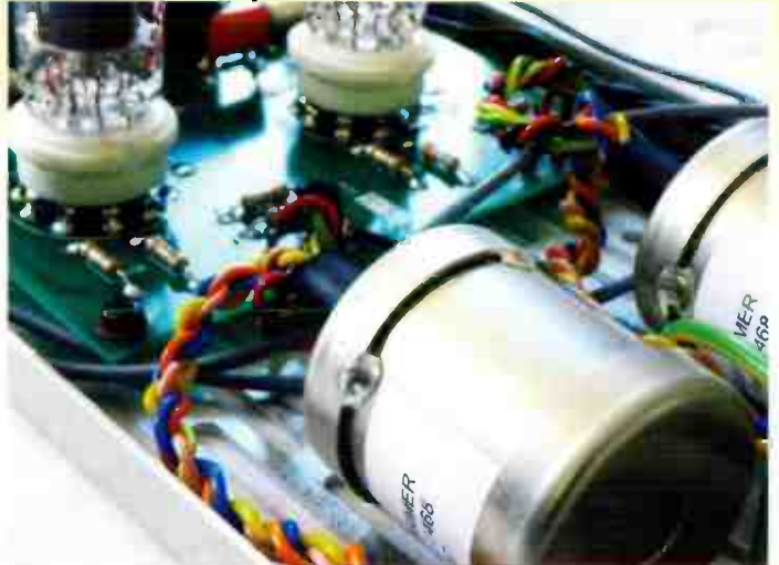
WDPhono3 prototype with MCT step-up transformers fitted.
