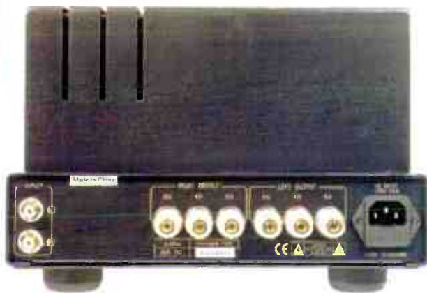
The Prologue 4 power amp., with 4ohm and 8ohm terminals.
