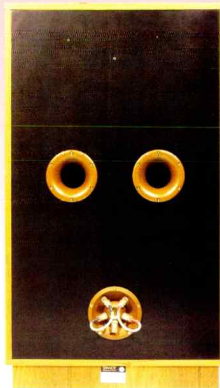
Two large rear ports signify this is a reflex cabinet. Tannoy fit a large bi-wire terminal set, able to accept very heavy cables and 4mm banana plugs. There is a terminal for an earth wire too.
