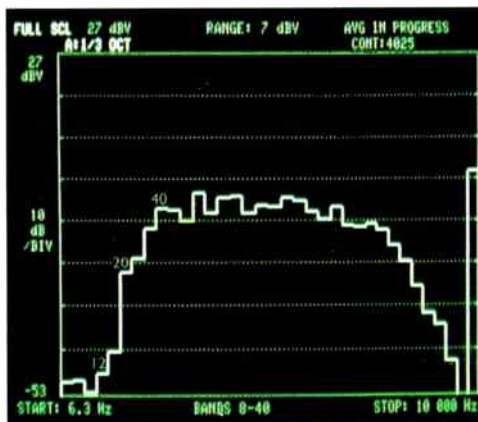
A typical music energy spectrum on CD. This analysis runs from 6Hz up to 10kHz. There is strong energy down to 20Hz.
