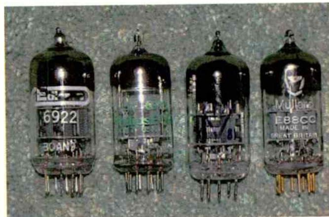
Fig. 4 Some E88CC / 6922 Valves: Edicron, Philips, Russian Navigator, Mullard New Shield and Mullard Old Shield Logo
