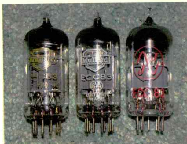
Fig. 2 Three of the ECC83s: Mullard Yellow Logo, Mullard White Logo and JJ
