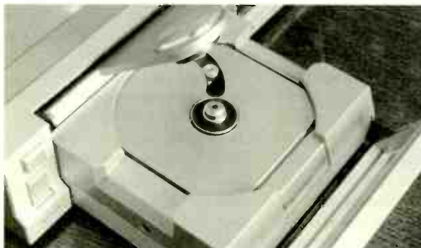
ye olde Philips CDM0 swing arm CD mech - shame all today's machines use cheapo DVD-ROMs..
