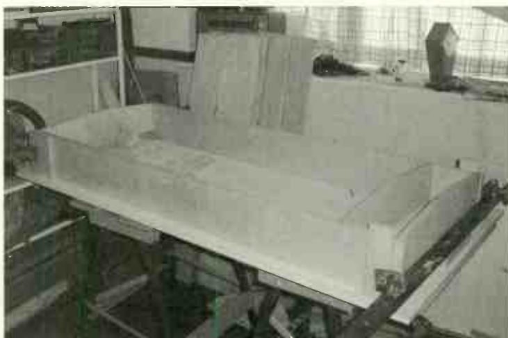
Cab Glue: cabinet all glued together.
