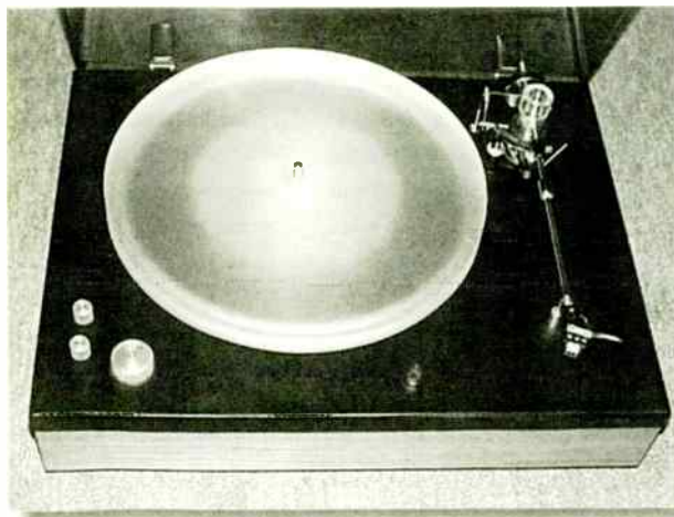
Here's the completed turntable, with acrylic platter. To the right is a Mayware unipivot arm, and to the left the speed controls that were retained.
