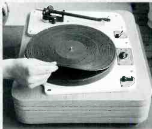
Removing a rubber or felt mat from a turntable's platter will affect the stylus's Vertical Tracking Angle.
