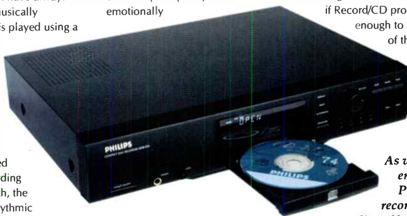
CD-R machines like Philips' CDR 870 produce digital copies almost identical to the originals, but analogue recordings tend to lose some of their character.
