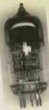
The 6922 valve may have been designed for RF circuits but it is perfectly suitable to audio use.
