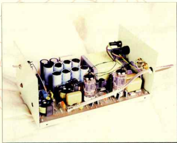
Inside the E. A. R. decoder. Here you can clearly see the valves which handle the mono signal.
