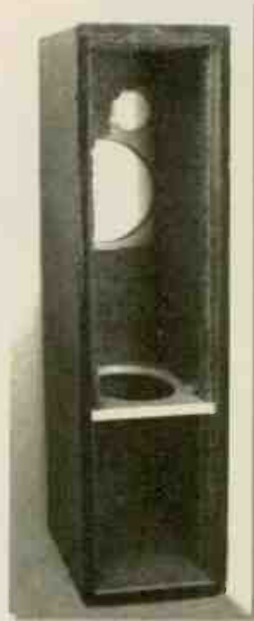
The inside view of the cabinet shows the bracing panel and damping pads. The cutout size is not critical, but should be big.
