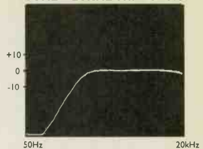
The 400Hz filter allows weak signals to be measured when hum and its harmonics are present.
