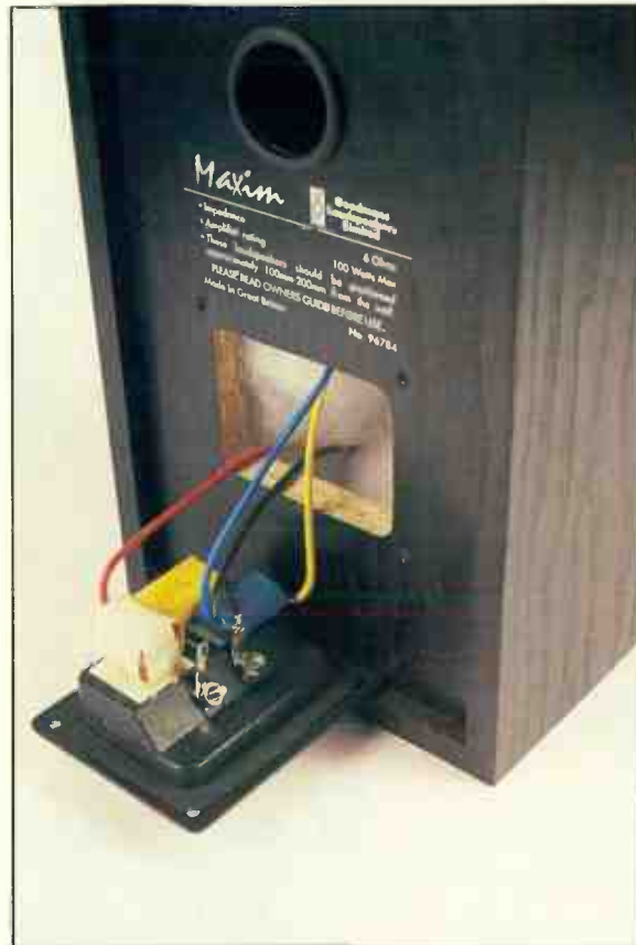
◀ Note the new blue and yellow capacitors that give a much more detailed treble than the electrolytics used in the Maxim 3s.
