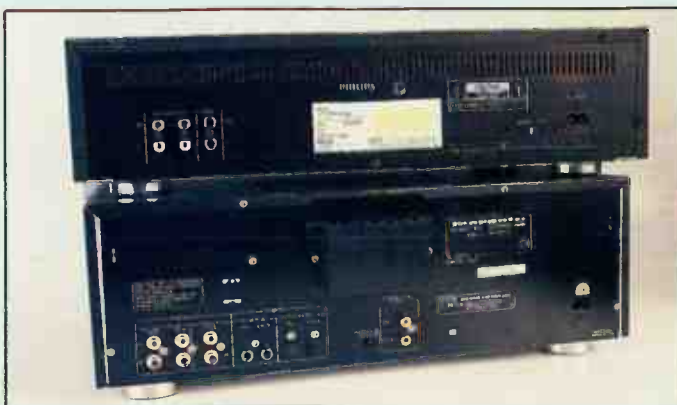
Both have coaxial digital and analogue sockets, but only the Marantz has optical.
