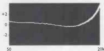
Steep high frequency lift gives sharp treble at normal bias (+3dB)
