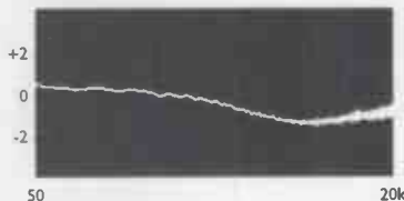
Raised bias (+4.5dB) subdues treble and improves dynamic range, but response cannot be tuned flat
