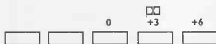
Fig 1 - Budget or mid-priced recorders usually have 0VU set below Dolby level, indicated by the Dolby sign
