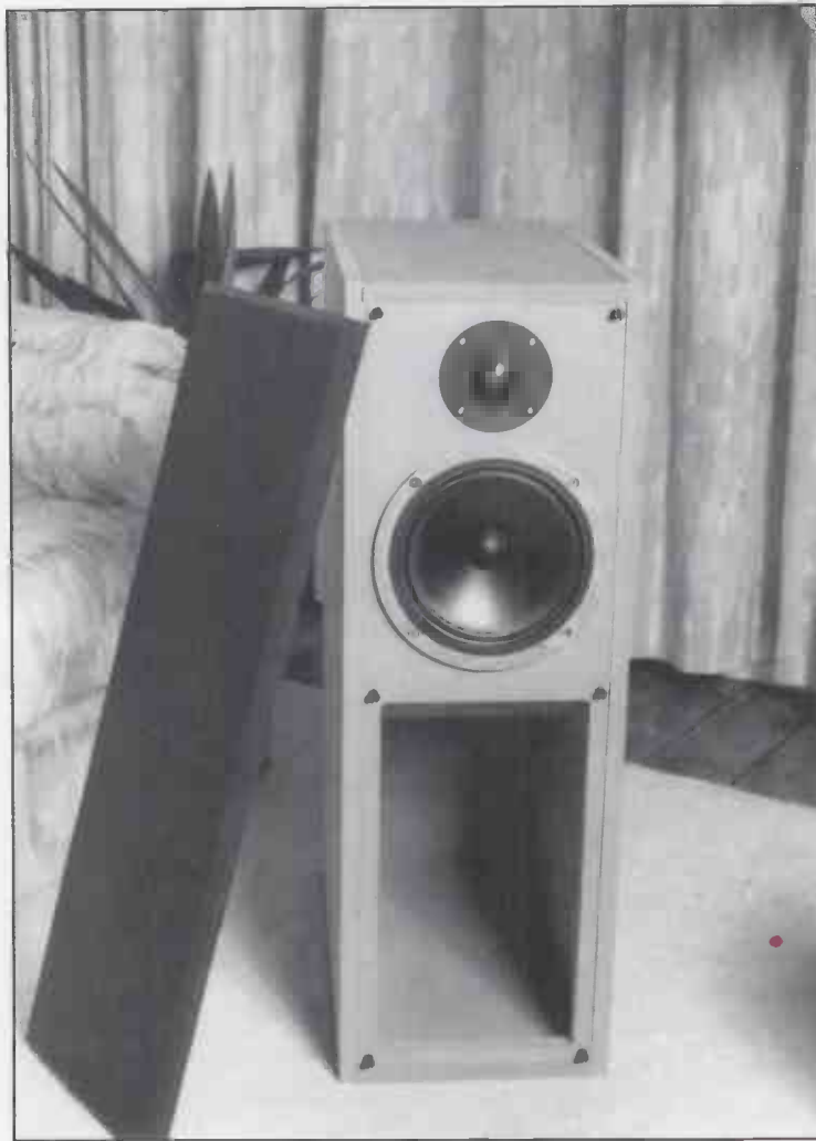
The assembled horn loudspeaker with its grille off
