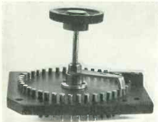
Fig. 6.—The inductance selector switch, mounted beneath the panel.
