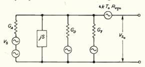
Fig. 11. Equivalent circuit for coupled circuit input.
