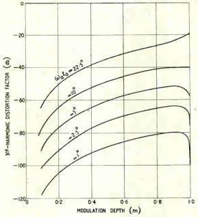
Fig. 2. Variation of 3rd-harmonic distortion factor with modulation depth and delay time.
