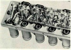
Fig. 9. Input stage of typical unit using capacitance neutralization—circuit used in 1946.
