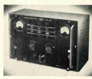
THIS unit provides a stabilised direct voltage, continuously variable from 200-350 volts, which may be used with either the positive or negative lines earthed, or with the output floating. An unstabilised alternating supply of 6.3 volts, the centre top of which may be strapped to earth, is also available.
