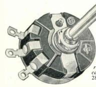
Conservatively rated at 3 watts; available up to 100,000 ohms linear. Diam. 1.21/32 in. Depth of case: 25/32 in. Spindle diam. 1 in. (insulated), Length to specification. Mechanical 300°. Effective 280°.
