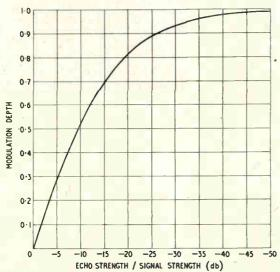
Fig. 3. Largest modulation depth for which analysis is valid.
