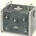
Susceptance: Equivalent to  $\pm$  75 pF to  $2^{\circ}_{0.5}$ , 0.5 pF Conductance: 0-100 mmho to  $\pm$   $2^{\circ}_{0.5}$ , 0.1 mmho
