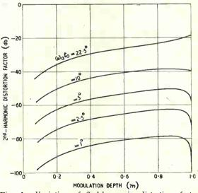
Fig. 1. Variation of 2nd-harmonic distortion factor with modulation depth and delay time.
