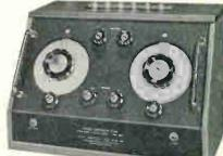
FOR BALANCED AND UNBALANCED MEASUREMENT FROM 15 KC/S -5 MC/S
