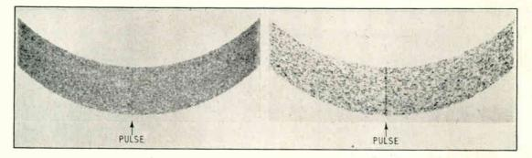
Fig. 8. Chemical recorder traces comparing 'linear' and coherent detectors; pulse duration = 2 ms; white-noise background of 500-c/s bandwidth; input signal/noise ratio (i.e.,  $R_1$ ) = 0.8 (- 2 db) for both types of detector.—N.B. This is 12 db below the ratios used in Fig. 6 thus showing the benefit of pulse-to-pulse correlation.
