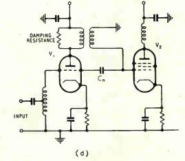
Fig. 8. Neutralized circuits. (a) Resonance neutralizing feeding pentode. (b) Resonance neutralizing feeding common grid. (c) Capacitance neutralizing with auto-transformer. (d) Capacitance neutralizing with conventional transformer.
