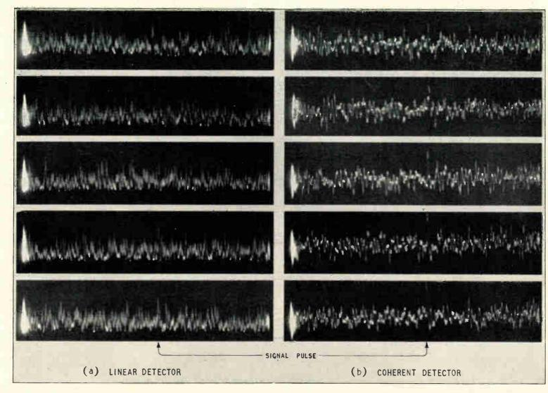
Fig. 7. Photographs of single traces on cathode-ray A-scan display; pulse duration = 2 ms; white-noise background of 500-c/s bandwidth; input signal/noise ratio (i.e.,  $R_1$ ) = 3 for both types of detector. For each type of detector 5 single scans are shown, chosen at random.
