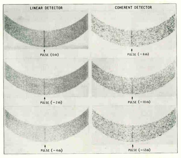
Fig. 9. Chemical recorder traces comparing 'linear' and coherent detectors on the basis of equal output signal/noise ratios; pulse duration = 5 ms; white-noise background of 500-c/s bandwidth; input signal/noise ratios for 'linear' detector 0, -2 and -4 db, for coherent detector -8, -10 and -12 db. It can be seen that the coherent detector gives detection at an input signal/noise ratio about 8 db lower than that required in the 'linear' detector.
