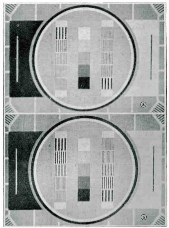
Fig. 5. These photographs show part of a television picture of Test Card C. The signal has been degraded by passing it through a 2-Mc/s  $\pi$ -section low-pass filter with the result depicted at (a). The use of 1st-, 2nd- and 3rd-order derivative correction is illustrated at (b).
