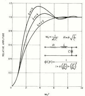
Fig. 4. Indicial response of simple low-pass filter.
