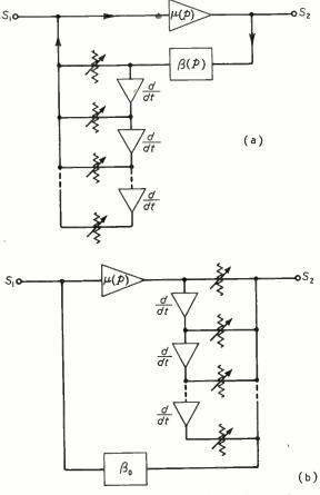
Fig. 3. Equalization of (a)  $\beta$  path and (b)  $\mu$  path.
