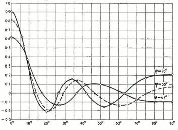
Fig. 7. Diffraction pattern of 1-high 6-wide array at different elevations; spacing  $r = 5\lambda/2\pi$ .
