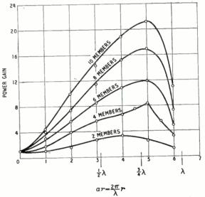
Fig. 2. Power gain of curtain of long filaments relative to single filament.
