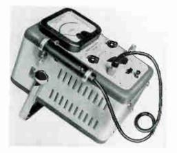
Furzchill sensitive valve voltmeter covering 1 mV to 100 V in five ranges; the frequency range is 10 c/s to 500 kc/s and the meter scale is logarithmic.
