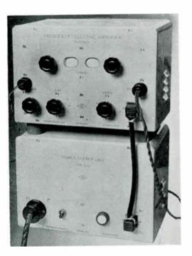
Tinsley frequency-selective amplifier and power unit, type 5212, covering 10-10,000 c/s with a Q of 32-35 and 80-100-db gain.
