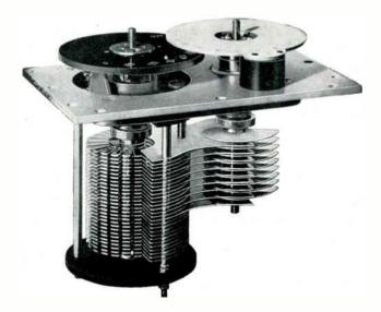
introduced in a manner such that small angular movements, due to a possible uncerfainty of click positioning, produce only very small edge capacitance changes on one sector only—in no position is there the slightest change of coincident active plate area.
