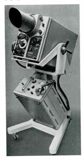
Nagard oscilloscope, type L 103, on adjustable stand with its power-supply unit.
