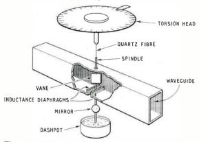
Fig. 1. Elliott waveguide power-measuring device.
