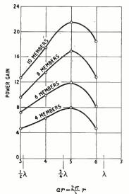
Fig. 5. Power gain of curtain of half-wave aerials relative to single half-wave aerial.
