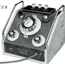
The Wayne Kerr Inductance Meter uses a stable variable frequency oscillator to resonate the unknown inductance with a known capacity. Calibration and scale reading accuracy are sufficient to give direct reading within  $\pm 2\%$  for values above  $1\mu$ H and relative measurements can be made with even greater accuracy.
