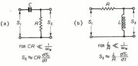
Fig. 7. Basic differentiating circuits.
