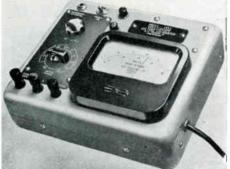
(above) Cossor model 1433 voltage calibrator for oscilloscopes.
