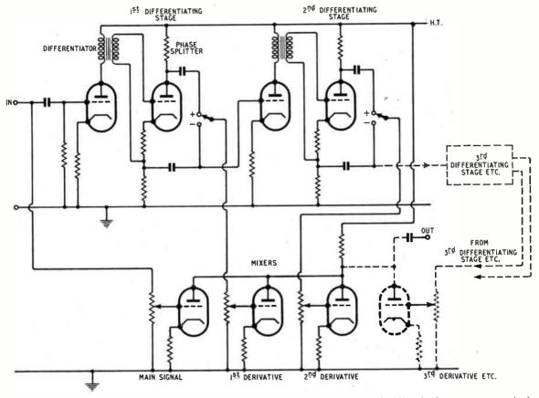
Fig. 10. Simplified circuit diagram of 2-stage wideband equalizer showing method of adding further stages as required.
