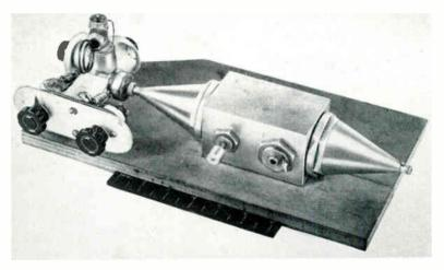
Fig. 2. Impedometer and Standards Unit.
