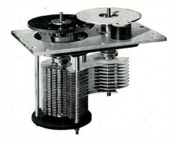
introduced in a manner such that small angular movements, due to a possible uncertainty of click positioning, produce only very small edge capacitance changes on one sector only—in no position is there the slightest change of coincident active plate area.
