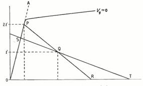
Fig. 6. Basic pentode characteristic.
