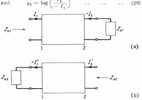
F: 2. Iterative propagation function of network driven at end 1(a), and driven at end 2(b).
