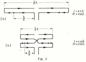
experiments were made with the dipoles horizontal and only about 25 ft above the ground; as  $\lambda/2$  was about 35 ft, it is probable that the results were appreciably affected by the proximity of the ground. The input resistances are from 20 to 30% above the calculated values; the highfrequency resistance of the wires constituting the dipoles is only about 1% or less of the measured values and can be ignored.
