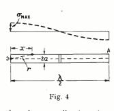
simple dipole а of length  $\lambda/2$  and exaggerated radius a. At the moment of zero current the charge is distributed according to a cosine curve as shown. We wish to calculate the potential at O, the point centre of one end, due to the charge, allowing for retardation, that is
