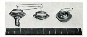
Fig. 5. Directional couplers for 30-60 Mc/s (left) and 50-100 Mc/s (right).
