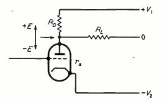
Fig. 2. Direct-coupled stage equivalent to Fig. 1.
