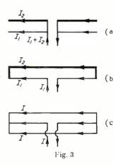
current I the power input is 73  $I^2$ , and if the single wire is (a) replaced by two wires of different diameters so that the current in one is  $I_1$ , and that in the other  $I_{2}$ , the (b) radiated power will be 73  $(I_1 + I_2)^2$ . If now the two elements of the dipole are arranged as in Fig. c) 3(b), so that the current is only supplied directly to one and induced in the other, for the same
