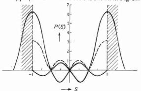
Fig. 12. Component patterns of the polar diagram of the aerial of Fig. 11.
