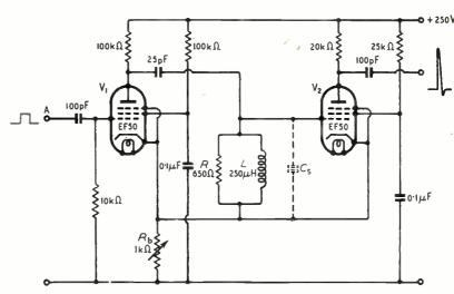
Fig. 4 (right). Circuit arrangement of cathode-coupled flip-flop pulse generator.
