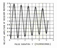
Fig. 4. Variation of amplitude with pulse duration.
