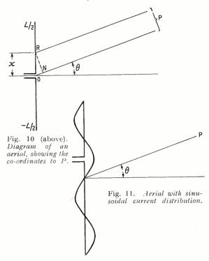
Since, in the frequency spectrum case we found that the unit pulse was a useful fluctuation with which to deal, we shall use its equivalent here and shall begin by calculating the polar diagram of an aerial of length L over which the current has constant unit value, and outside which the current is zero.
