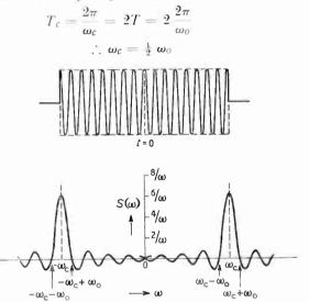
Fig. 2 (above). Pulse modulate l by a cosine wave. Fig. 3 (below). Component spectra of the pulse of Fig. 2.
