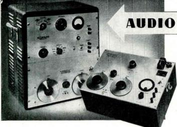
Laboratory Standard B.F.O. Type L.O. 800 and Portable Model L.O. SO.
