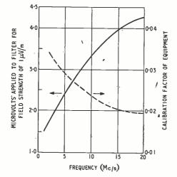
Fig. 3. Pick-up factor of aerial and calibration factor of equipment; aerial length 6-1 m.
