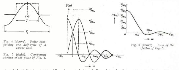
placed about the t = 0 axis. All we have to do is to draw on transparent paper two identical patterns representing the spectrum of a pulse (Fig. 1), superimpose them, and displace by the required amount, centring the spectra on  $\pm \omega_c$ , and add the overlapping portions in the positive half of the frequency plane.
