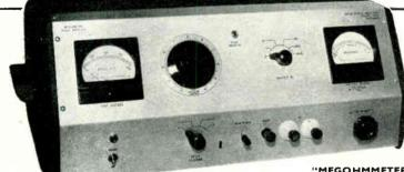
Designed for the measurement of high values of insulation resistance as experi-enced in modern materials and electrical components. Completely self-contained components. Completely self-contained and mains-operated, providing its own D.C. test pressure. All essential voltages stabilised, giving constant readings even with fluctuating mains voltages as experi-enced under industrial conditions. industrial
