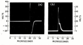
Fig. 6. Typical voltage pulses showing effects of varying cathode-bias resistance  $R_{b}$ .
