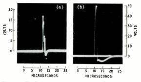
Fig. 7. Typical voltage pulses showing effects of varying coil inductance L.
