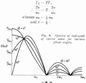
We now evaluate (12) with  $x = \frac{1}{2}$  for different values of  $\phi$ . The result is shown in Fig. 9. We notice, as is to be expected, that as the function changes from a half-cycle with a maximum at t = 0 ( $\phi = 0$ , half-cycle of cosine wave) to a halfcycle with zero at t = 0 ( $\phi = 90^\circ$ , half-cycle sine wave), the d.c. component becomes progressively less and the amplitude of the higher frequency components progressively greater.
