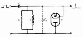
Fig. 1. Production of a short pulse from a sudden positive-going voltage change, with the aid of a highlydamped oscillatory circuit.
