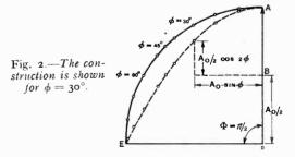
OA to OE, it does not agree strictly with equation (2). Instead of following the circular arc it follows the curve shown. A closer approximation would be obtained by making the carrier amplitude somewhat larger than  $A_0/2$  thus raising the whole curve. To get accurate agreement, however, the amplitudes of the components must be obtained from a table of Bessel functions,
