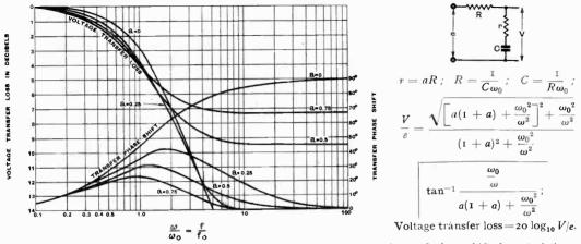
Fig. 6.—Circuit for increasing  $\pi$  attenuation with generalised attenuation and phase shift characteristics.
