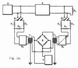
now be of the constant impedance type, the circuit constant being adjusted so that  $T_1$  and  $T_2$  always work between the same impedances as one another.
