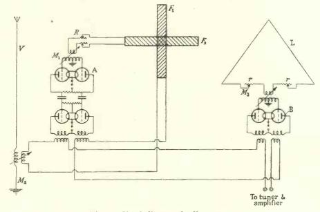
Fig. 4.—Circuit diagram of radio compass.
