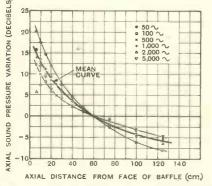
Fig. 6.—Axial sound pressure variation with distance for constant loudspeaker current.
