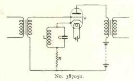
transmitter or a heterodyne whistle on the lowfrequency side, a rejector circuit L, C is inserted in the cathode lead of an indirectly-heated value V, shown in the Figure as a low-frequency amplifier. A resistance R supplies grid bias.
