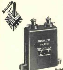
The Dubilier Type BB Condenser is a high-efficiency condenser in moulded bakelite case. Working voltage 200 D.C. (peak. Test, voltage 400 D.C. Capacities from.09 mfd to 4.0 mfd. Prices 1/9
