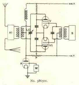
until the output from the valve V commences to "droop," whereupon it contributes the required extra energy to the common output circuit LC feeding the power amplifier  $A_{I}$ .
