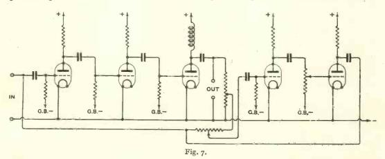
The theoretical limitation of this circuit is, of course, that it is only the output stage, not the whole amplifier, which is compensated, so that the distortion introduced by the first two stages remains without reduction.
