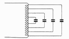
Fig. 1. Condensers representing the self capacity of an inductance coil.
