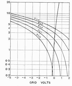
Fig. 9. Logarithmic grid characteristic diagram, with portion of Edison D.R.2 characteristic.
