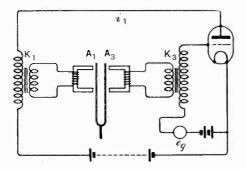
Fig. 7. To illustrate mechanical consideration of valve-maintained tuning fork theory. False factors  $A_1$  and  $A_3$ .
