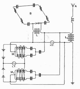
vertically polarised wave, and from a loop aerial Bwhich produces a horizontally polarised wave. High frequency oscillations from the source HF are transferred alternately through a magnetic modulator  $M_1$  and coupling  $L_1$  to the aerial A, and through a second modulator M and coupling L to the loop B, the frequency of the change-over being controlled by a low frequency alternator LF.
