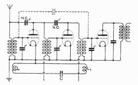
any other subsequent valve, so that at least two stages of valve amplification separates the two coils. The condenser C has a capacity of  $0.006\mu$ F. As shown the closed coupling-circuit is connected to the filament system.
