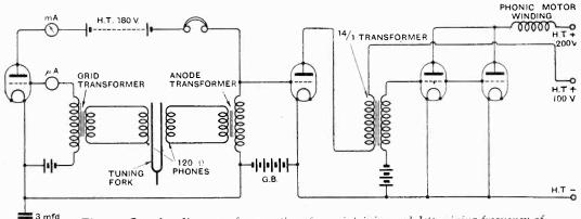
Fig. 9. Complete diagram of connections for maintaining and determining frequency of maintained-tuning fork.
