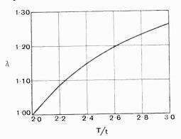
Fig. 10. Graph for determining the initial rate of rise of temperature from the average rate of rise.
