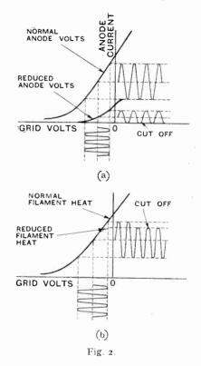
valve is asymmetrical and that only one halfcycle is markedly susceptible to curvature in the valve characteristic.
