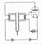
Fig. 1. Simple circuit of valvemaintained tuning fork.
