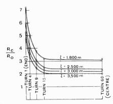
Fig. 11. Distribution of loss in experimental coil.
