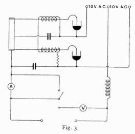
as read on moving iron instruments, and has now been in use for two years charging for 24 hours each week. The only renewal necessary has been that of the mercury every three or four months, and the initial cost apart from that of the condenser and meters was nothing.
