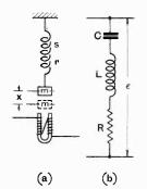
Fig. 6. (a) Mechanical analogy. (b) Electrical analogy.
