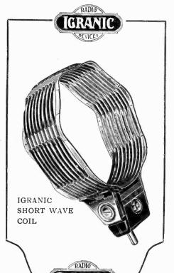
The success of a short wave receiver depends to a large extent upon the ability to produce and control oscillation. The design of Igranic Short Wave Coils, the low self-capacity and minimum H.F. resistance enables oscillation to be obtained easily. Igranic Short Wave Coils are wound with heavy gauge wire, rigidly supported with a minimum of insulating material, which accurately preserves the spacing between turns. Igranic Short Wave Coils are made in four sizes for wavelengths of 10-100 metres.
