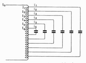
Fig. 5. Approximate circuit assumed for a long coil at high frequency.
