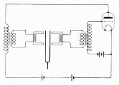
Fig. 2. Circuit of valve-maintaining tuning fork using transformers.
