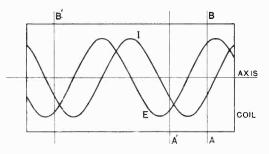
Fig. 7. Showing distribution of current and voltage on a very long coil.
