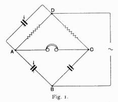
At low frequencies, where bridge methods of measurement can be used, there should be no difficulty in using a guard ring and keeping it at the potential of the insulated electrode. Thus in the equal armed bridge, Fig. I, the guard ring can first be connected to A and then to C. Let  $C_1, C_1'$  be the readings of the condenser in the arm AB, and  $C_0, C_2$  be the capacities of the guard ring
