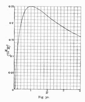
clearer idea of the nature of the problem. If the "open circuit" E.M.F. of the battery is e volts, its internal resistance  $R_0$  ohms, and the resistance of the load R ohms, then the current will be
