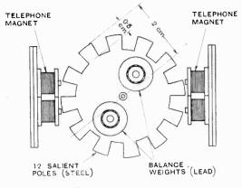
Fig. 10. Diagram of synchronous motor.
