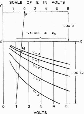
Fig. 12. Chart relating the quantities E, V and  $v_A$  to G, the slope of the logarithmic characteristic. The point P corresponds to E = 2; the point Q corresponds to V = 3.88,  $v_d = 1.34$ . The gradient of PQ is that of the characteristic shown in Fig. 9; the horizontal and vertical scales of Figs. 9 and 12 being in a fixed ratio.
