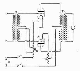
two tappings being taken to selected points on the resistance  $R_{p}$ , forming the source of the plate voltage. It will be seen that both resistances  $R_g$  and  $R_p$ , together with the two valve filaments, are all in series across the terminals of the supply mains M.
