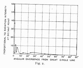
azimuth. This radiation intensity for various angular deflections is plotted graphically in Fig. 2.
