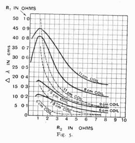
We give, by way of example, in Fig. 5 the results of measurement of the frequency of 1,130,000 cycles (265.5 metres wavelength).
