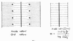
and v = -3, also the same anode current is obtained with V = 100 and v = -6, so that if V is increased by 20 volts v has to be decreased by 3 volts.
