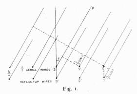
The magnetic field of each wire is propagated as a wave, and is also inversely proportional to the distance. Therefore at a distance  $\gamma$  and time t may be considered to be proportional to  $\frac{I}{\gamma} \sin(m\gamma - nt)$  where  $m=2\pi/\lambda$  and  $n=2\pi/T$ . T being the periodic time and  $\lambda$  the wavelength.
