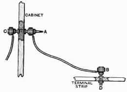
Fig. 33. All the outside connections are made to the cabinet, and short flex leads go thence to the baseboard.
