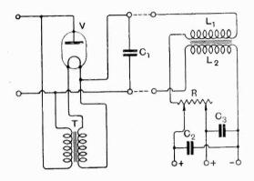
manner, and an integrating condenser  $C_1$  is connected before the chokes. The remainder of the filter circuit is constituted by another condenser  $C_2$  across two chokes  $L_1$  and  $L_2$  in each lead respectively.
