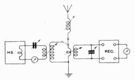
by the receiving signal, as indicated by the meter in the output of the receiver. Then knowing the ratio of transformation of the current transformer it is possible to determine antenna currents which do not allow of direct measurement.
