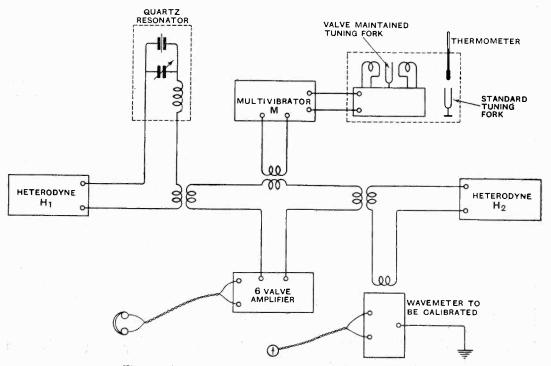
Fig. 6. Circuit arrangement used for wavemeter calibration.
