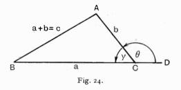
The vectors c=a+b, a, and b form a triangle as shown in Fig. 24.
