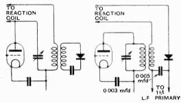
Fig. 26. This is a more satisfactory reaction arrangement than that of Fig. 25, but it is still by no means the best. Fig. 27. Here we have the reaction circuit finally adopted, which proved very satisfactory.
