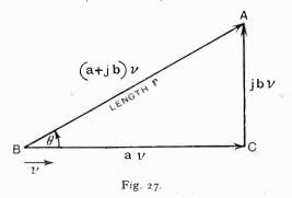
which make  $\theta$  quite definite for given signs and magnitudes of a and b. The effect of the operator (a+jb) is thus seen to be a rotation through  $\theta$  specified as above, combined with a multiplication by  $r = \sqrt{a^2 + b^2}$ , and this effect is quite independent of the actual operand, which may be a unit vector as in Fig. 27, or any other vector whatever. Further by a suitable choice of a and b, r and
