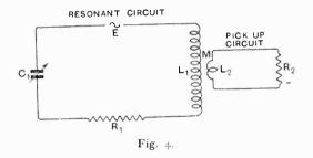
We will call E the effective electromotive force in the resonant circuit; we will say that it is constant, seeing that in principle the reaction of the wavemeter on the transmitting station to be measured should be negligible.
