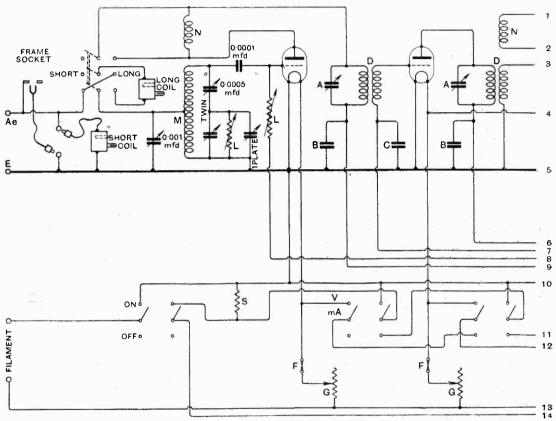
Fig. 29. The complete schematic diagram. In order to make this fairly easy to read, it has been increased in size. Note that the numbers given to each wire at the break correspond with one another. The values of components are given in some cases in the drawing, the remainder are as follows: A,  $0003\mu F$  max.;
