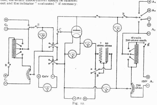
2. To secure low power consumption and independence of frequency the grid should be connected directly to the circuit to be measured, and ample bias used.
