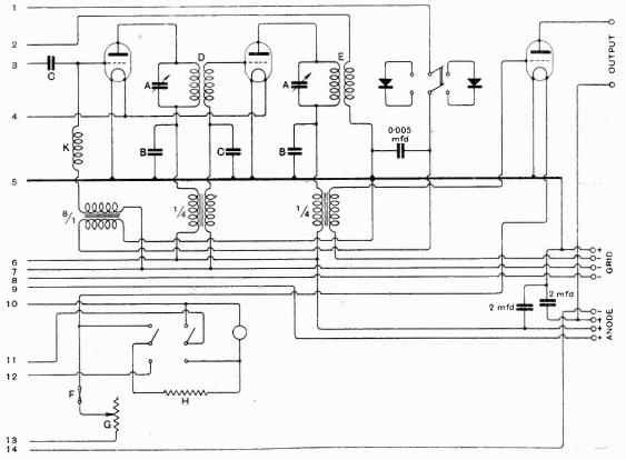
B,  $003\mu F$ ; C,  $0003\mu F$ ; D, McMichael air-core, No. 3; E, As "D." but secondary rewound to  $\frac{1}{2}$  turns; F, Burndept fixed resistor in holder; G, Filament rheostat; H, Series resistor for meter; K, 1.800 or 1,500 coil of low self-capacity; L, Variable leak, 1–5MO; M, McMichael "Autodyne" unit; N, McMichael reactor.
