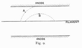
I mm. diameter connected by molybdenum cross piece. The filament takes 50 amps at 20 volts, giving an emission of 7 amps and in assembly is slid into the anode so that one leg of the filament lies axially in each chamber of the anode.
