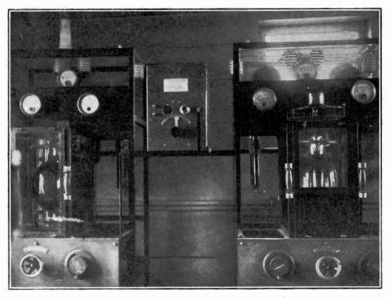
Fig. 9. Showing the standard wavemeter installed in the Radio-Belgique station at Brussels.
