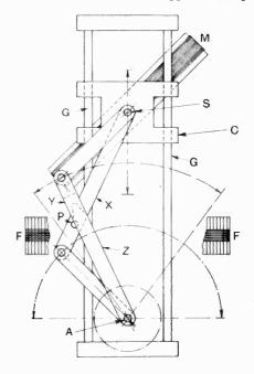
in the link arm X engages a guide plate Y on the link arm Z, and carries it over the top dead centre in a direction depending upon the rotation of the spindle A.
