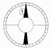
Fig. 42. For checking bearings: a large compass card, set by means of a small compass and then locked. The actual card is of course marked in degrees.
