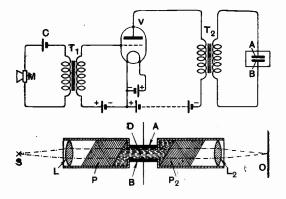
light to change in intensity. Since the rotation of the plane of polarisation occurs simultaneously with variation of voltage that is, there is no lag, the device is readily applicable to television purposes.
