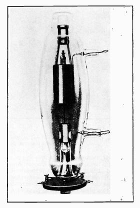
Fig. 4. Short-wave transmitting value for about 1.5kW.
