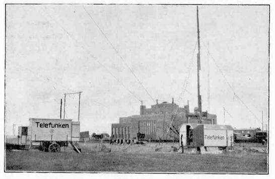
Fig. 8. Transportable short-wave transmitter POF.
