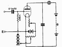
Fig. 32. Connections of the slide back voltmeter, Type V., using a grid condenser and leak.
