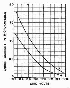
Fig. 27. Anode current—grid bias curves, in the region of zero anode current, for two slightly different A.C. voltages.
