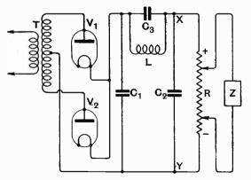
$V_1$  and  $V_2$ , the values being used for full wave rectification in conjunction with a centre tap on the secondary of the transformer. The output of the rectifier is taken through a form of  $\pi$  filter comprising two condensers  $C_1$  and  $C_2$ , on either side of an inductance L shunted by a capacity  $C_3$ . Normally, the load, such as the current used by a
