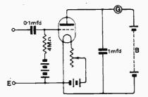
Fig. 29. Connections of the deflecting voltmeter, Type IV., rectifying on curvature of the anode characteristic but using a grid condenser and leak.
