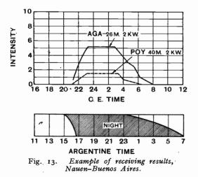
the POY transmitter, which worked simultaneously with AGA and transmitted on a wave of 40 metres with an output of 2kW.
