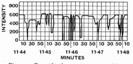
Fig. 12. Example of reception, disturbed by fading effect.
