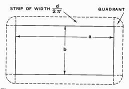
Fig. 3. Showing the effective size of a rectangular condenser plate.
