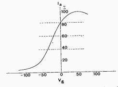
Fig. 10. Curve showing the relation between the aerial current and the grid voltage of the modulating valve.
