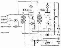
Fig. 21. Connections of the transmissionmodulation meter.
