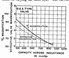
Fig. 9. Showing decrease in magnification with increase in capacity at a given wavelength, the inductance being gradually reduced as the condenser is increased (D.E.3 valve).
