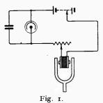
The new method is explained here as it is carried out in co-operation with a modified form of the wellknown flashing circuit of the neon lamp described by Pearson and Anson (*Proc. Phys. Soc.*, p. 204, 1922).
