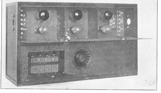
Fig. 13. Three-stage microphone amplifier.
