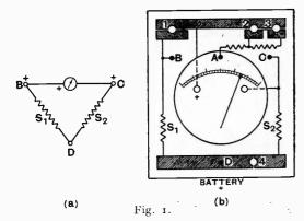
When charging, the accumulator  $S_2$  is in series with the ammeter whilst  $S_1$  is shunted across them. When the battery is being discharged through the filaments  $S_2$  becomes the shunt across ammeter and  $S_1$  in series.
