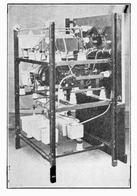
Fig. 12. Back view of panel for control of main anode and aerial currents.
