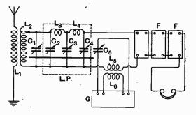
reception employing a low pass filter. The specification mentions that with ordinary heterodyne reception it is possible to obtain more than one adjustment of the local oscillator for any desired beat note, thereby resulting in confusion.
