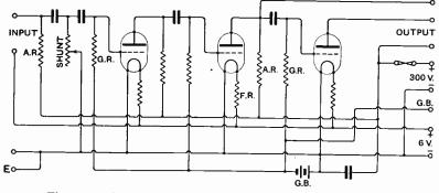
Fig. 14. Connections of the 3-stage microphone amplifier.
