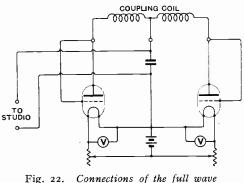
Fig. 22. Connections of the full wave rectifier.
