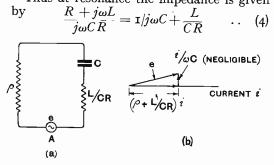
Fig. 7. Showing that at resonance the tuned anode combination is equivalent to a condenser C in series with an inductionless resistance L/CR, the whole being in series with E.M.F., e and valve resistance p.
