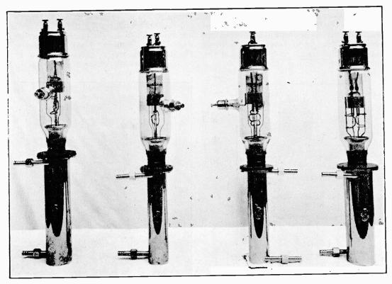
Fig. 9. Water-cooled power value RS204.
