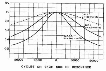
Fig. 11. Curves showing gain in selectivity with a large condenser across tuning coil.
