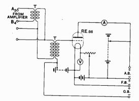
Fig. 18. Connections of the amplifier modulation meter.
