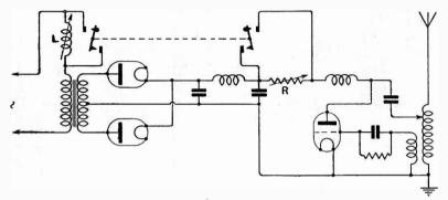
Fig. 4. Another keying circuit which produces a spacing wave.
