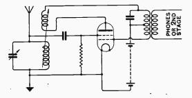
also illustrated, the transformer secondary in this case working to the outer grid of the succeeding valve, with arrangements similar to those shown in its inner grid and anode circuits. Only the usual four-electrode valve H.T. of about 12 volts is required and it is stated that excellent results have been obtained on both near and distant transmissions.
