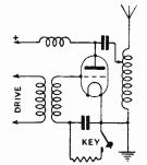
Fig. 6. Method suitable for small power transmitters using an independent drive.
