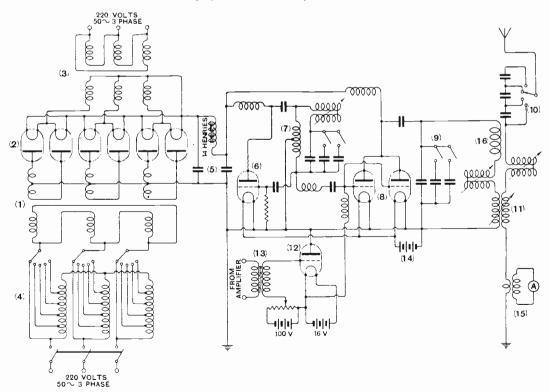
Fig. 6. Connections of the transmitter. The numbers in brackets are explained in the list at the foot of the next page.
