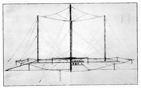
Fig. 4. Schematic view of aerial and counterpoise.
