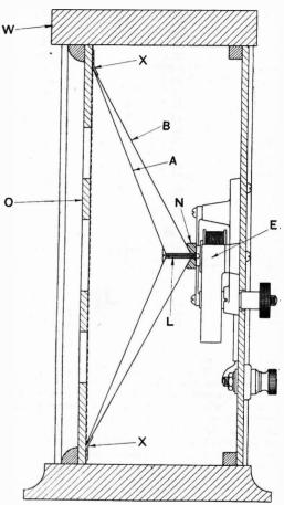
plug N to which they are joined by a screw L. This screw communicates with an ordinary electromagnetic system E, such as a telephone receiver, which is used to energise the cones. It is stated that the cones may be made of paper, parchment, thin wood, or metallic foil.
