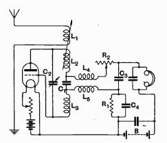
circuit contains an inductance  $L_1$ , tightly coupled to a split inductance  $L_2$   $L_3$ , tuned by a variable condenser  $C_2$ , the split inductance being connected by a fixed condenser  $C_1$ . Inductance  $L_4$  and  $L_5$ constituting the inductance of the quenching circuit, are associated with a condenser  $C_3$ . The lower
