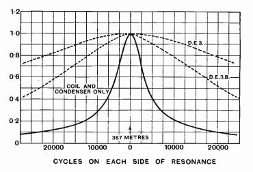
Fig. 10b. Showing relative selectivity curves of tuned anode with and without value damping.
