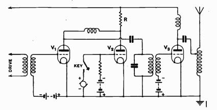
Fig. 9. Keying method applicable to high power transmitters.  $V_1$  is the intermediate magnifier,  $V_3$  the main magnifier, and  $V_2$  the absorbing values.
