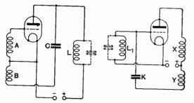
is connected directly between the anode and the H.T., and the other winding Y is connected to the grid through a capacity. Here, again, the capacity K forms the major portion of the capacity in shunt with an inductance  $L_1$ , connected, of course, this time in the grid circuit. This circuit should prove of interest to experimenters, and it is found to be very satisfactory in practice.
