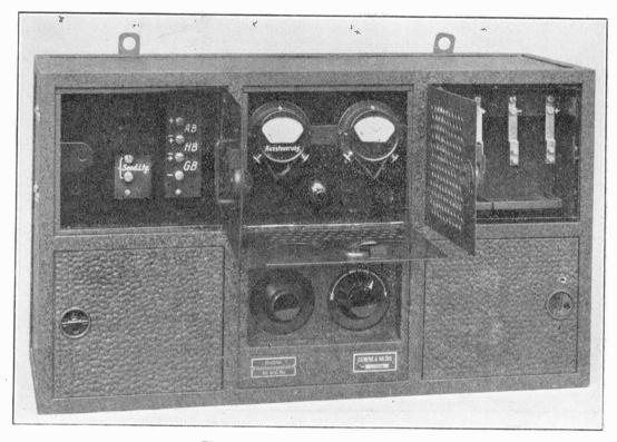
Fig. 17. Amplifier modulation meter.
