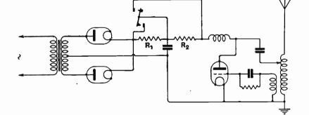
Fig. 3. A keying circuit in which the value can oscillate weakly during the spacing intervals.
