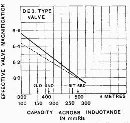
Fig. 8. Showing decrease in magnification with increase in wavelength (due to increase in capacity of anode tuning condenser). Calculated for D.E.3 value for which m = 7 and  $\rho = 22,000$  ohms.
