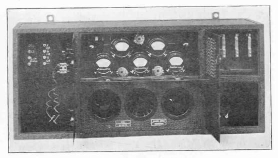
Fig. 19. Transmission-modulation meter.
