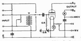
Fig. 16. Connections of the additional 4th stage amplifier.
