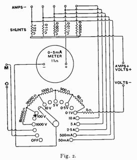
The internal connections of the test set.
