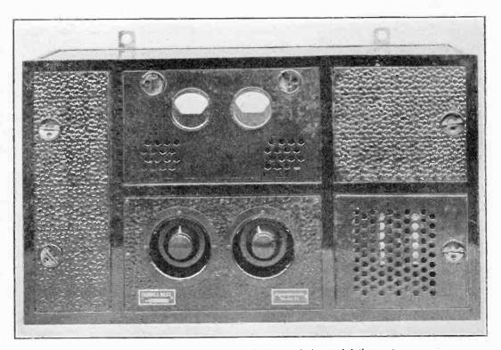
Fig. 20. Full wave rectifier operating transmission-modulation meter.
