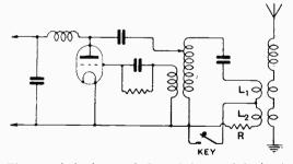
Fig. 5. A keying method used in coupled circuit oscillators.
