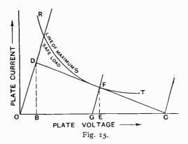
We can obtain greater efficiencies by increasing the resistance of the output circuit and raising the anode voltage as shown in Fig. 15 where DFC is working line.
