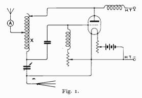
the radio-frequency choke employed in the shunt feed circuit. The removal of this choke probably has the effect also of sharpening the tuning-always a desirable feature.
