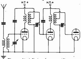
Fig. 2. Aperiodic transformer couplings.
