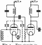
Fig. 1. Two circuits in cascade employing the neutrodyne principle.
