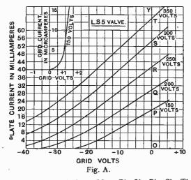
two columns of the table. P', Q', R', S', T' correspond to P, Q, R, S, T of Fig. A. By taking a series of values of  $E_g$  (—10, —20, etc.) and going through a similar process we obtain the complete
