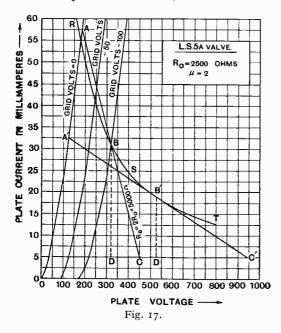
For  $R_{\epsilon} = 2R_{0}$  the working line giving 10 watts loss is *ABC*. This gives an A.C.
