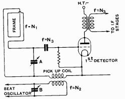
Fig. 3. Theoretical diagram of superheterodyne.
