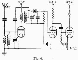
Convenient circuit for using a crystal with one H.F. value stage neutralised followed by L.F. stages.
