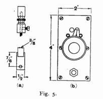
block to facilitate adjustment of the bobbin to give a spot at central zero. However, setting is not troublesome as it stands.
