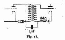
the effect of the arrangement is roughly to increase  $\sigma$  to  $(\sigma + 1)$ . Results of measurements, shown in a tabulation, reveal a fairly flat-topped curve of amplification.
