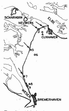
The results are tabulated on the next page. Here K stands for coast station, and L for inland station. The measurements show no effect of the level of the water on the intensity or direction of the radio waves, nor can any change of intensity be detected with certainty as the waves pass from water to land. In any case the change cannot be great. It thus appears to make no perceptible difference to the propagation of waves whether
