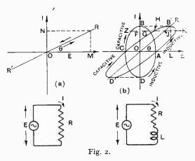
Case (B). Pure Inductance.  $E=L\omega I$  but I lags 90° behind E. The locus is composed of two simple harmonic motions at right angles and in quadrature. This locus is an ellipse ABCD traversed in the counterclockwise direction, as this makes the maximum of I lag 90° behind that of E.
