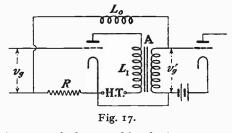
resistance of the graphite leak type. The arrangement gives a good range of constant amplification, experimental results on this point being shown in a table. The circuit is quite workable in practice. If R be increased, a setting is reached where oscillations cocur
