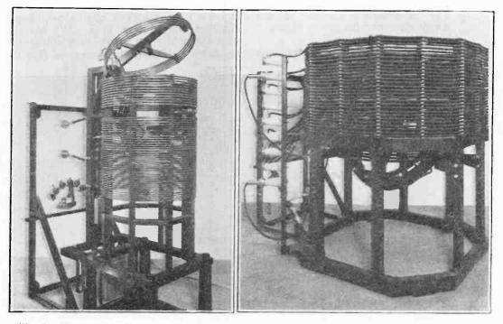
Fig. 8. Main anode coil and aerial coupling.
