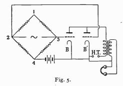
obtained. Earth balance is effected on the Wagner principle by the variable resistance and  $C_0$  and measurement finally adjusted. With  $S_1$  and  $S_2$  in their lower and right-hand positions respectively, the connections of Fig. 6 are given for final measurement of
