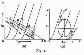
If the external load comprises resistance and inductance in series the equation showing the relation of the changes in  $e_p$  and  $i_p$ becomes.
