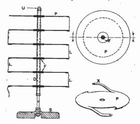
Durrant and K. I. Rayment. Essentially the aerial consists of a number of plates of appreciable area, supported co-axially one upon the other. Thus, in the accompanying illustration, a stand S is provided with an upright member U which
