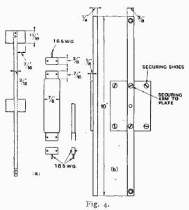
obtained and carefully marked out as shown in Fig. 4 (a). A sharp knife was used on the narrow parts and shears with extreme discretion on the end pieces. Two small rivet holes were made to coincide and tiny lead rivets used for fixing.
