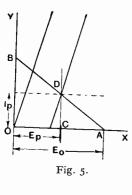
ourselves to sinusoidal conditions, it is clear that the AC power output will be a maximum when the working range extends from A to B, Fig. 3b. Тο secure this with ideal characteristics, the grid bias should make D the mean position, the mid point of AB. (See Fig. 5.)
