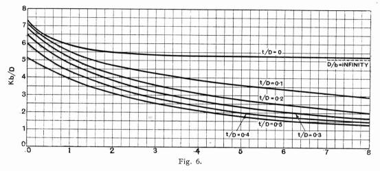
stitutes the final solution of the A.C. resistance problem for solid wire coils with well spaced windings.
