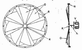
that although the diaphragm is formed of a number of sectors which vibrate more or less as a whole,' owing to the fact that the sectors are combined rigidly near their point of actuation the maximum flexibility occurs at their extremities.
