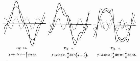
and amplitude a/3, beginning in phase with the fundamental. It is now very noticeable that the half cycles are each symmetrical and mutually similar. There is also evident the beginning of a flat top, referred to later.
