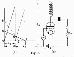
For the other type of circuit (Fig. 8b) altering  $R_e$  does not change the conditions in the valve so long as there is no alternating. voltage on the grid. Hence in Fig. 8 when  $R_e$  only is altered the working line will swing about D, and the grid bias would have to be altered to make the working line pass through A.
