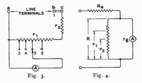
When using the instrument direct, the link between terminals b and c is opened, and the flexible lead from one side of the ammeter is connected to terminal b (No. 1). For other ranges, it is connected to terminals 2, 3, 4, etc., and the link between b and c is replaced.
