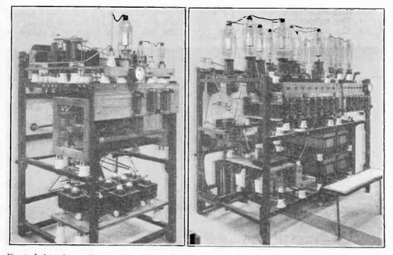
Fig. 6. Independent oscillator and modulating valves.
