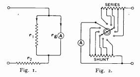
instrument when used by itself, and in order to secure this condition we shall have to insert an extra resistance in series with the combination. Consider now the circuit shown in Fig. I. Let  $R_t$  be the total resistance between the line terminals under the new conditions. July, 1926
