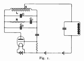
R and condenser  $C_1$ . Variation of  $C_1$  varies the energy consumption in R, and therefore the damping of LC. A further condenser  $C_2$  is preferably placed across the damper to compensate for change of tune,  $C_1$  and  $C_2$  being varied in opposite senses so that their total capacity remains constant. The controls of tune and of reaction are said to be practically independent of each other over a large tuning range.
