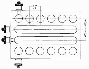
Fig. 11. A simple type of connecting board.
