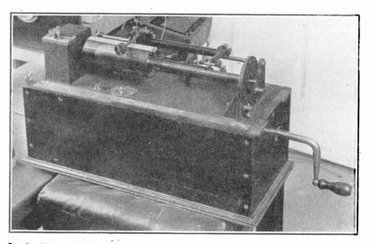
In the Thorne Baker picture transmitting apparatus a copper plate bearing the image is traversed by a metal needle forming part of an electrical circuit. The receiving and transmitting equipments are exactly similar, and the cylinder on which the picture is recorded by an electrolytic process is kept in synchronisation with the transmitter by means of accurately-timed pendulums.
