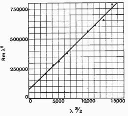
Fig. 5. Showing how A' and B' in the formula  $R_m = \frac{A'}{\sqrt{\lambda}} + \frac{B'}{\lambda^2}$  (26) may be found by plotting  $R_m \lambda^2$  against  $\lambda_s^8$  and finding the slope (A') and the intercept on the vertical axis (B') of the resulting straight line.
