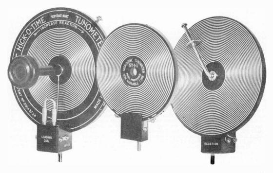
wound in spiral grooves cut in both faces of an ebonite disc. In the first three coils tuning is effected by a rotating arm carrying a small grooved wheel which runs on the wire, and as the arm is rotated the number of turns of the coil in circuit is altered. The arm and wheel are held in good contact with the wire by means of a fairly strong spiral spring concealed in the long bearing for the arm.
