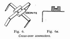
Fig. 6 shows a cross-over connector, Fig. 6a showing the method of mounting. A small square of ebonite about  $\frac{1}{4}$  in. thick has one limb fixed to the under side, the other being fixed to the upper side, which is better recessed to take it, so as to keep it well insulated from the body when handling. The ends of all connectors should be amalga-
