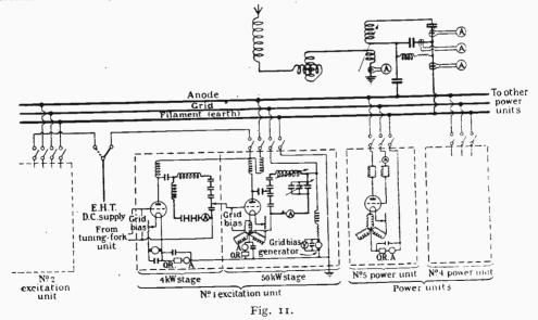
Fig. 10 is a skeleton diagram of the circuit arrangements from the output of the tuningfork unit to the aerial. The tuned highnecessarily generated by a valve transmitter when operated as an efficient power amplifier, and thus acts as a desirable harmonic filter. Fig. 11 is a schematic diagram showing the method of feeding the H.T. D.C. supply through a selected excitation unit to the
