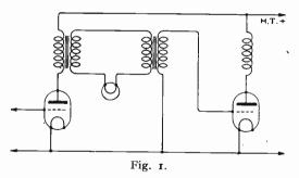
1.5 ohms when cold (or under very small applied voltages), and in the neighbourhood of 16.5 ohms when 3.5 volts are applied to it. The essentials of the scheme are shown in Fig. 1. The actual modulation arrangements used at Radio Toulouse are also illustrated, several lamps being used in parallel.
