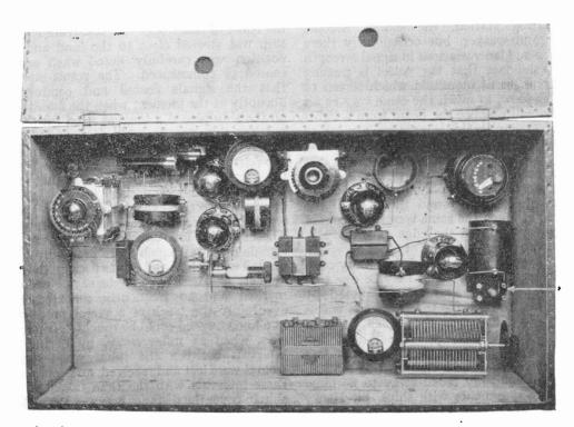
The photograph shows an American crystal controlled transmitting set. The master oscillator (driven by the crystal) operates at 209.4 metres, and the fifth harmonic (41.88 metres) of this is amplified in succeeding values until the desired output is obtained.
