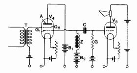
electrode valve, which is associated with the usual loud-speaker and batteries. The invention states that the overall magnification approximates to an inverse function of the frequency, and is very high for audio-frequencies. It is further stated that the 334
