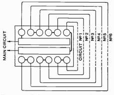
Fig. 12a. Indicating the method of inserting connectors with all circuits in series.
