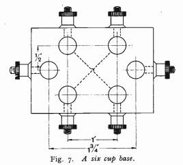
tors, so that circuits can be put in series or parallel or disconnected at will. Using the double connector it becomes a double-pole switch in either direction, and with the twoway cross-over it can be employed as a reversing switch.
