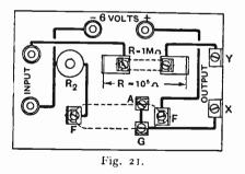
$R_2$ , is included in the filament circuit, both to limit the current through the valve and to counteract the effect of the electron pressure. This resistance is wound with No. 26 D.C.C. Eureka wire, and is adjusted until, with the input terminals shortcircuited, the reading of the microammeter connected to the "hooks" X and Y (Fig. 21) is just reduced to zero.
