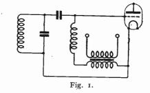
the "stopping condenser" and radio frequency choke to keep the H.F. component out of the L.F. transformer. The complete circuit of Fig. 2 is then shown, where the "stopping condenser" is shown, dotted at the filament end of the H.F. circuit. The following values are given ;---
