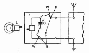
that the tuned circuit comprising L and C can be connected to the set in more than one position.
