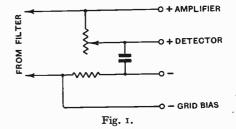
opposite half cycles to give double wave rectification. The ionised gas is Argon. Output curves are given, for output current against voltage. The usual type of filter is illustrated giving output tappings, as shown in Fig. 1, for the provisions of intermediate H.T. to the detector and for gridbias.
