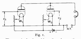
The method of making the observation may conveniently be considered in relation to Fig. I. Here  $W_1$  and  $W_2$  are two valves, the filaments of which are controlled by separate rheostats. The anodes of these valves are connected in parallel through a pair of telephones and a source of H.T., and values have linear characteristics and identical mutual conductances and if  $v_1$  and  $v_2$  are equal and in opposition of phase then no sound will be heard in the telephones.
