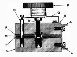
Between these is interposed a sheet of dielectric M of mica or similar material. The ends of the two plates are brought out and fixed to terminals provided with soldering lugs L. The two blocks are provided with threads of different pitch, a central rod R also provided with two differently pitched threads being placed between the two blocks. A locating pin N is screwed into the lower block. The end of the rod R is provided with
