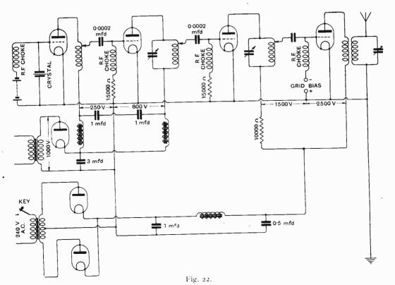
A set of this type may be modulated in any of the usual ways. Whichever method is used there will be no chance of frequency modulation. Modulating the grid of the last amplifier is a very simple and satisfactory method. In other circuits this usually gives so much frequency modulation that the telephony is unintelligible, but using this method with crystal control many
