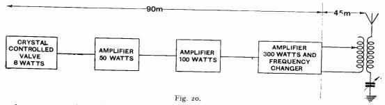
only one stage of amplification is used. It is the addition of the second and third stage necessitating a frequency change and the accompanying losses that reduces the overall efficiency of the set.
