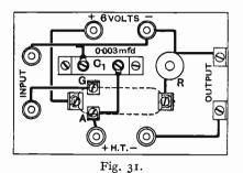
actual instrument is the "D.E.V." Although really intended for 3 volts, it works quite satisfactorily on 2 volts and is then, of course, very unlikely to change or "burn out." It is probable that the "D.E.Q." valve would be still more suitable as it is especially made for "anode rectification."
