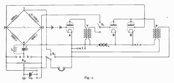
to the grids of the values are applied alternating voltages  $v_1$  and  $v_2$  from any source whatever. Then it is clear that if the voltage amplification of a valve and transformer is illustrated in Fig. 2, which is a simplified circuit diagram of the test set.
