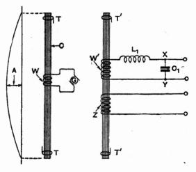
A suitable reception aerial and its associated circuits is shown on the right of the illustration. Similar short-circuited turns  $T_1$  are shown for the purpose of tuning, and a similar winding  $W_1$  is
