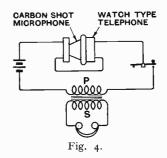
It should be added that the foregoing circuit should be successful with D.C. mains, as the commutator ripple is usually sufficient to actuate it.
