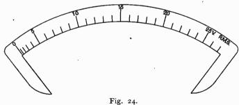
case where the microammeter scale is not "direct-reading." Cut out a piece of stout paste-board to fit the glass-covered opening of the microammeter case, shaping it so that only the scale of the instrument is covered. Then mark upon this card the
