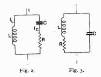
Fig. 2 shows a rejector circuit consisting of a condenser of capacity C in series with a resistance R, shunted by an inductance L.
