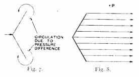
at the side very many of the high tones have disappeared, but at the front they are felt in full force. With a cone loud-speaker in the open, where there are no reflections, the beam effect is more pronounced.
