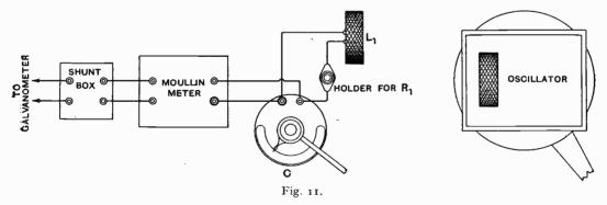
Here then in Fig. 11 is the layout used by the writer. On the right is the source, an ordinary valve wavemeter with about 60 volts on the anode. It is mounted on a wooden turntable, for reasons which will appear later.
