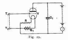
It is this grid bias that fixes the upper limit of the A.C. voltage that can be measured. Under the above circumstances, its peak value must not exceed four volts, or, in other words, its R.M.S. value must not exceed  $4 \times 0.707$ , say, 2.8 volts.
