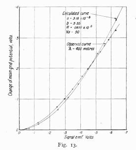
lengths of 400, I 000 and 4000 metres. In every case the variation with frequency was small, probably less than the limit of accuracy of the measurements.
