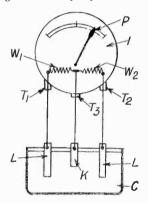
and it will be seen that the device consists essentially of a differentially wound voltmeter provided with two ordinary terminals and a third terminal connected to an auxiliary electrode designed to be introduced into the electrolyte of the cell to be tested.
