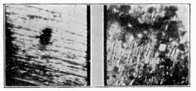
Fig. 4. A piece of natural galena polished to a high degree of brilliance on a polishing lap.
