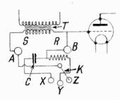
such as condensers or resistances shunted across the secondary of a transformer, which is connected to the input of a low frequency amplifier valve. The specification contains actual constructional details of a device of this nature consisting of
