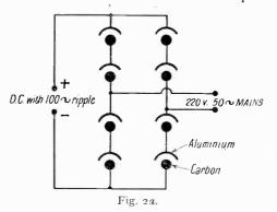
light up fully for a moment and then slowly die out. When the lamp is extinguished, forming is complete, and if the operation is performed in a dark room, the electrodes will appear to be covered with a luminous sheen.
