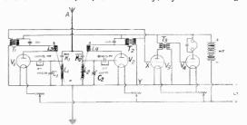
some speech frequencies at one radio frequency, while the others are transmitted at another radio frequency. The present invention consists in providing a receiver which will respond simultane-
