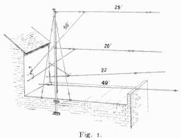
aerial systems. This allows for transmission and reception on short waves and the simultaneous reception of broadcast programmes in another part of the house. The transmitter does not interfere with the broadcast programme being received although situated so near to the receiver.
