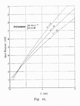
4. For a given grid-circuit resistance the input resistance increases with the signal amplitude, but the increase is relatively small.
