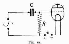
acting in a circuit of external resistance R. In general  $E_{\epsilon}$  depends chiefly on the amplitude of the alternating E.M.F., but also to a less extent on R. The effective internal resistance  $R_{\epsilon}$  also depends to some extent on both the alternating E.M.F. and on R. The change of continuous potential difference across the resistance R is given by
