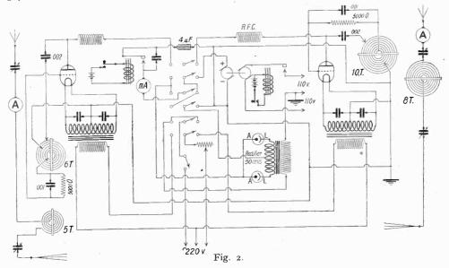
in an ebonite strip as shown. The values of the other components of the 40-metre set are shown in the diagram. The primary coil, like the aerial coil, is wound with  $\frac{1}{2}$ -in. brass ribbon and the inside turn has a 7-in. diameter.
