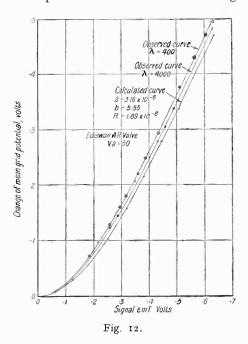
voltage characteristic of the valve was measured separately under the same experimental conditions of filament and anode voltage.
