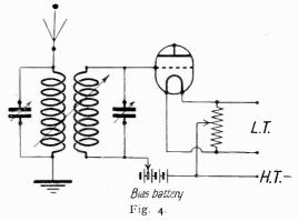
present if the latter method is used, and for fairly strong signals, anode rectification gives far superior quality. The connections for valve detection are given in Fig. 4.
