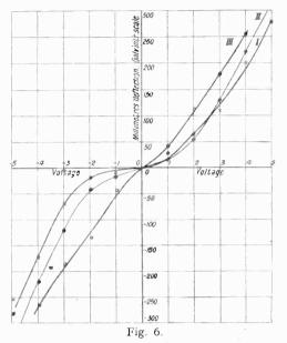
Characteristic Curves for the Crystals treated. Curve I: Good rectifying crystal. ,, II: Second grade crystal. ,, III: Poor crystal.
