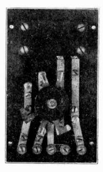
multiple switch shown, the variable condenser can either be connected in series with the aerial (first position), or a small fixed condenser (about '000 5) can be placed in shunt with the tuning inductance when on stud two. In position 3 (safety) aerial and earth are shorted, while the fourth places the variable condenser in parallel with the inductance-the fixed condenser being shorted.
