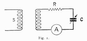
Further, as the closed circuit is tuned, its reactance is zero. Hence, if  $R_0$  is the resistance of the circuit itself, and  $I_r$  is the current in it
