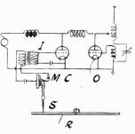
microphone M. The microphone M is connected to a stylus S, which is in contact with a gramophone record or similar device R. The invention relates
