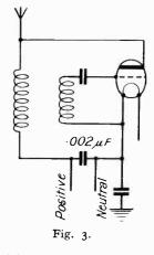
series with the positive or anode feed and will effectively remove the chance of a short circuit at the transmitter side of the supply. A 32 c.p. carbon lamp is as good as anything.\* If a lamp is
