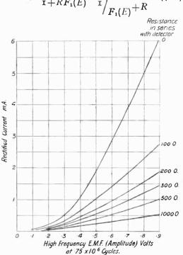
Fig. 9. Rectification characteristics for Galena with various loads.
