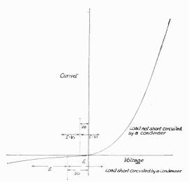
Fig. 7. Illustrating the effect of the load in diminishing the output.
