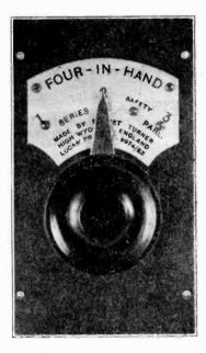
T is often verv useful to be able to switch over one's aerial condenser from series to parallel, but the advantage is trebled if by so doing an overlap in wave-length can be obtained without altering the aerial coil. This fact has been realised by Mr. Ernest Turner, of High Wycombe, who has patented an arrangement a back and front view of which is reproduced herewith.
