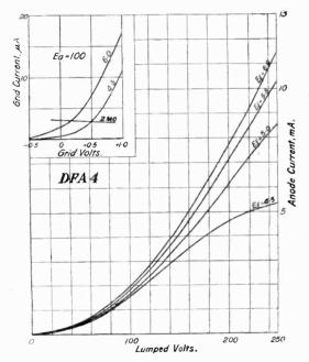
also rather below the average for valves with these filaments, being 30mA maximum instead of the usual 40. We are inclined to think that the filament of this sample had a resistance slightly above the average, and so was running cooler. The anode
