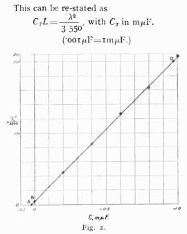
Now, if the self-capacity of the coil is  $C_s$ , and we make two tests with different values,  $C_1$  and  $C_2$ , of the condenser, giving  $\lambda_1$  and  $\lambda_2$ as wave-lengths, we have
