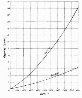
Fig. 14. D.C. output against square of H.F. input, for small inputs.
