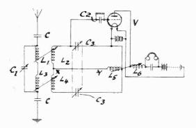
a reaction effect is obtained between  $L_2$  and  $L_6$  resulting in increased signals. Should oscillations be generated, it is stated that the currents being equal and of opposite phase in  $L_2$  and  $L_4$ , their combined induced effect in  $L_1$ ,  $L_5$  in the aerial circuit will be substantially zero, or in other words there will be no radiation from the aerial.
