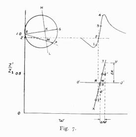
Join EP, and note the point M, where EP intersects HKL. Now choose some zero line below the original curve, such as O'O', and directly below the original point 2 set off R2'' equal to KM, above or below the zero line according as KM is above or below EG.
