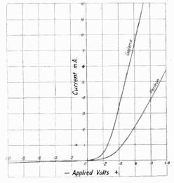
Fig. 1. The characteristics of two typical rectifying crystals.
