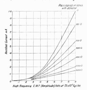
Rectification characteristics for Perikon Fig. 10. with various loads.
