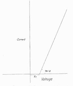
Fig. 4. At large amplitudes, the crystal characteristic approximates to a straight line.
