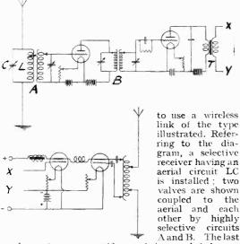
valve acts as a rectifier and is coupled by an output transformer T, which is connected at XY to the control valve of a low power transmitter. The system does not appear very novel to us, as we think similar schemes have been used prior to June, 1923. The idea of a wireless link, while being excellent from many points of view, always suffers from the effects of interference and atmospherics.
