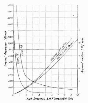
Fig. 15. Combined curves showing  $R_c$  and  $E_c$  for both large and small inputs.
