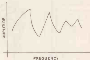
Fig. 1. The acoustic response of a room or other enclosure contains relatively sharp peaks and troughs.
