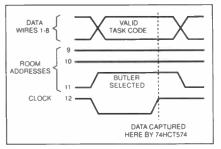
Fig.8.2. Command timing diagram.
