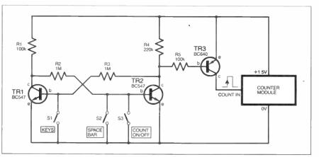
Fig.3. Typewriter word counter circuit.
