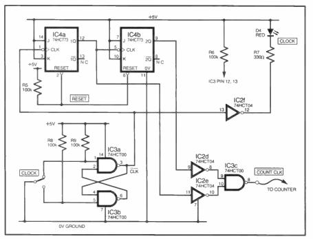
Fig.8.20. Assemble this Asynchronous 2-bit Counter, and link the  $\overline{Count CLK}$  output to the clock counter of Fig.8.19.
