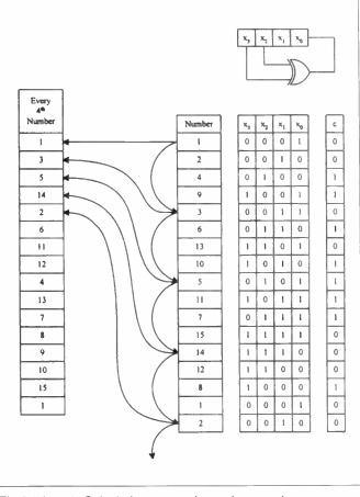
Fig.6 (above). Calculating a pseudo random number. Fig.4 (left). Main program state machine display flow chart.
