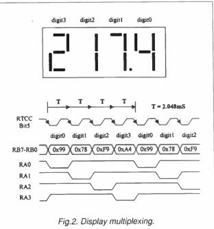
display. The display is made up by using two, dual-digit, modules X2 and X3. Whilst a four-digit version is available, the cost is more than that of the two dual modules.
