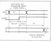
Fig.8.17. Flip-flop setup, hold times and propagation delay.
