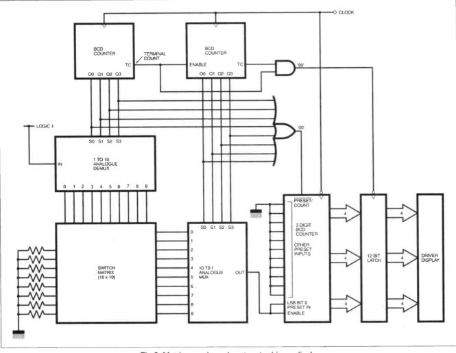
Fig.2. Matrix-scan based system to drive a display.
