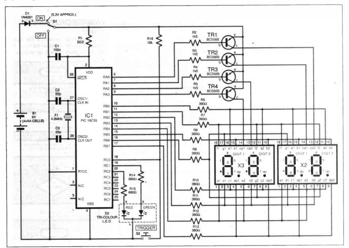
Fig.1. Complete circuit diagram for the Reaction Timer.
