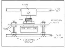
Fig.5. Suggested method of securing the Frequency control in the case.
