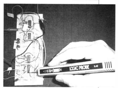
Using a logic probe to checkout our Lab Work exercise. The croc. clips are across the supply lines.
