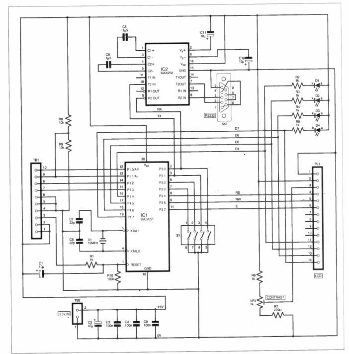
Fig.6. Circuit diagram for the Experimental Test Board.
