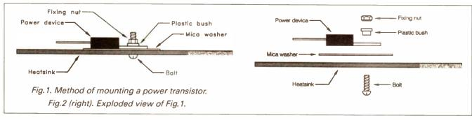
part of the circuit. you usually find that mounting a power device direct on the heatsink produces something like a short circuit on the output of a power amplifier or a short circuit across the power rails of the equipment.
