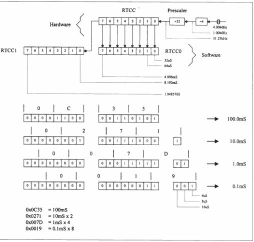
Fig.7. Calculating the reaction time.
