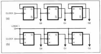
Fig.8.9. Asynchronous 3-bit binary up counters (a) using D-types, (b) using JKs.
