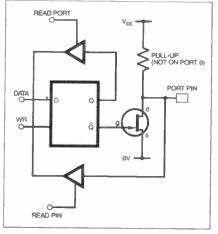
Fig.4. Typical port structure.
