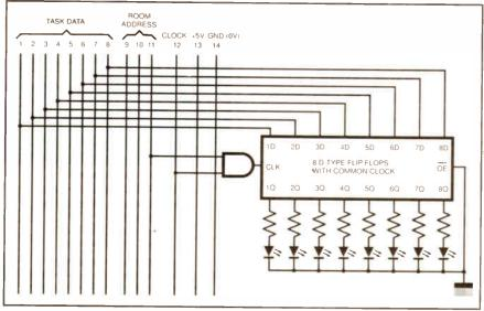
Fig.8.1. Command display circuit diagram.
