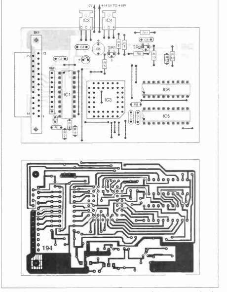
Fig.4. P.C.B. component layout and full size copper foil track master for the 2051/1051 programmer.
