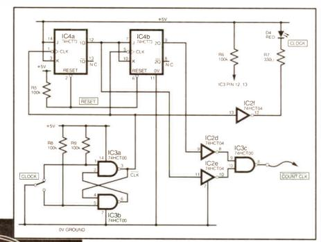
Fig.8.21. Modify the connections between IC4a and IC4b to form a Synchronous 2-bit Counter. wired together, and IC4b J and K inputs are connected to 1Q, the
