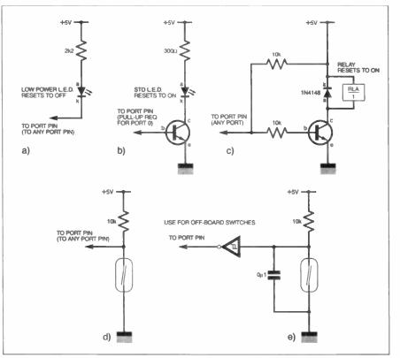
Fig.5. Examples of I/O drive circuits: (a) low current I.e.d., (b) buffered I.e.d., (c) relay drive, (d) simple reed relay, (e) improved reed relay.
