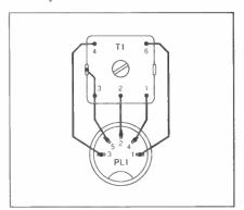
Fig.4. Pin connections from transformer T1 to the 5-way (180 degree) DIN plug.
