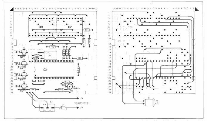
Fig.8. Stripboard component layout and wiring. Some of the interwiring on the underside is soldered **directly** onto i.c. socket pins and some component leads.
