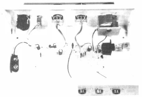
Completed Simple SW Receiver showing positioning of the circuit board and offboard components. Note the aerial and earth sockets are mounted on the rear panel.
