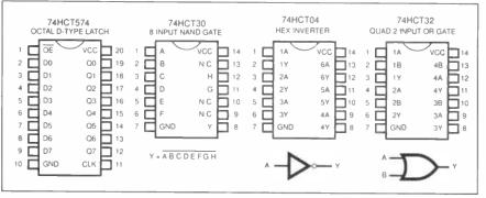
Fig.8.5. Pinout details for the chips used in the Household Command System circuit.
