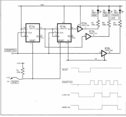
Fig.8.19. Construct this 2-bit Synchronous Counter to count clock pulses. Use RESET first, before commencing counting, and link COUNT CLK to the next two demonstrations.
