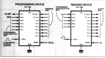
Fig.1. Signal routing for programming and reading the AT89C2051/1051 devices.
