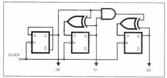
Fig.8.16. Another 3-bit binary synchronous up counter. This one uses the toggle/hold circuit of Fig.8.15
