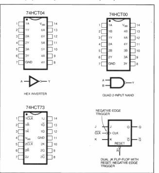
Pinout details for the MOS logic i.c.s used in the counter circuits.
