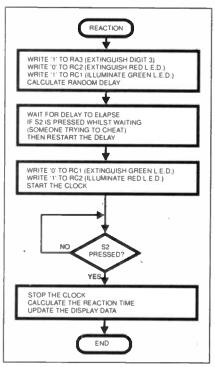
Fig.5. Software flow chart for reaction time.
