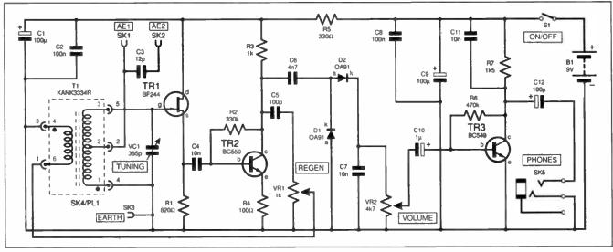
Fig.2. Full circuit diagram for the Simple SW Receiver. The numbers inside the unshaded area are for the plug-in r.f. transformer coils and those outside are for the 5-pin DIN socket.
