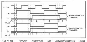
Fig.8.18. Timing diagram for asynchronous synchronous counters.
