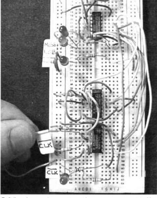
Building the synchronous/asynchronous counters, labelling the l.e.d.s and "toggling" the clock.
