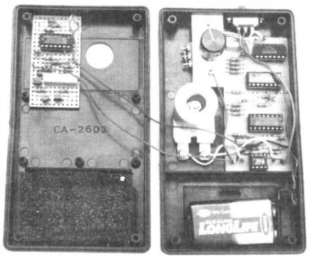
The two halves of the project case showing the component positioning. The small board in the case lid is the Low-Power L.E.D. Battery Monitor. to be described next month.
