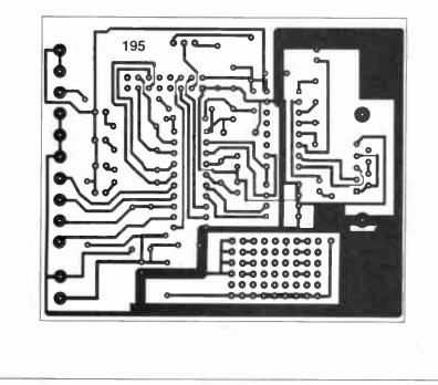
Fig.7. P.C.B. component layout and full size copper foil track master for the Experimental Test Board.
