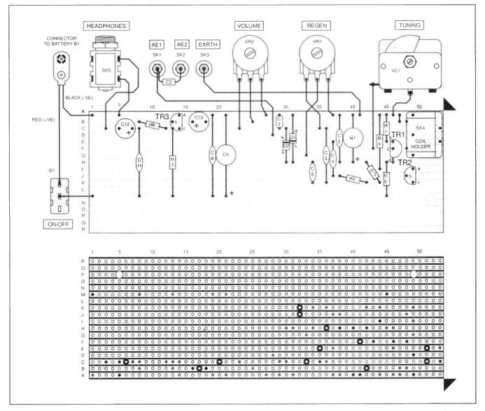
Fig.3. Stripboard component layout, interwiring and details of breaks required in the underside copper tracks. Note ALL copper breaks shown must be made.
