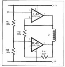
Fig.3. Modifying the output stage for higher power.
