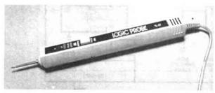
A useful piece of test equipment is the Logic Probe. The lead is terminated with a pair of crocodile clips.
