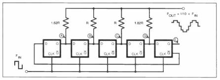
Fig.1. Simplified digital sinewave generator using D-type flip-flops.
