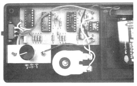
Completed unit showing components installed in the base of the case. Suggested methods for mounting the Frequency control and output coil are given in Fig.5. and Fig.6.
