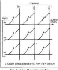
Fig. 1. 3 by 3 switch matrix.
