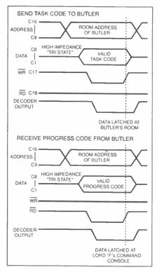
Fig.8.4 Read and Write timing diagrams for the Household Command System.
