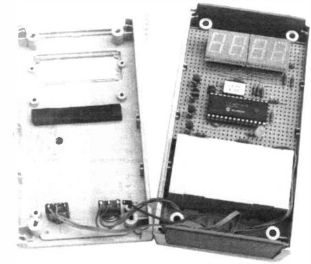
The completed Reaction Timer. The circuit board "sits" on the rubber strips glued to the sides of the case, at a height to allow the l.e.d. to protrude through the case lid.
