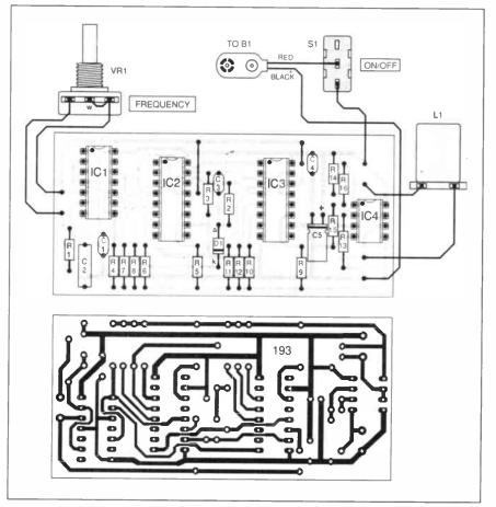
Fig.4. Printed circuit board component layout, off-board wiring and full size copper master pattern for the EPE Mood Changer.
