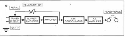
Fig.1. Block schematic diagram for the Simple SW Receiver.
