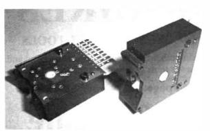
A typical "thumbwheel" switch. Using end cheeks on each side, they can be banked together.
