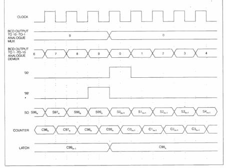
Fig.3. Timing diagram for circuit of Fig.2 (above right).
