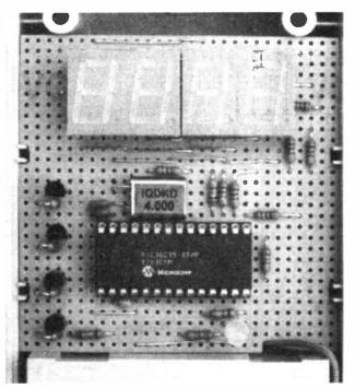
Component layout on the circuit board. Note the side cutouts to allow the board to slot into the case.
