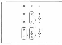
Fig.8.7. A  $1 \rightarrow 0$  transition on one bit causes the next significant bit to toggle.
