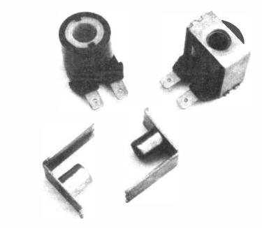
Producing an air-cored coil from a 230V solenoid coil salvaged from a washing machine three-way valve.
