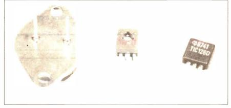
Various power transistors. From left to right the case styles are TO3, TO126 and TO220.
