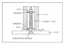
Fig.6. Coil mounting details.
