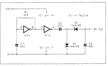
Fig. 3 The simple negative supply generator circuit diagram.
