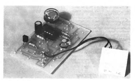
The completed circuit board showing connections to the relay coil. Connection to the relay contacts will depend on application.
