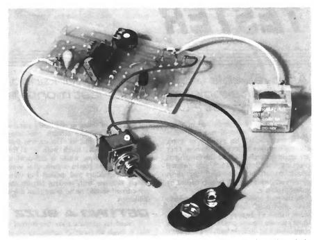
Wiring from the completed p.c.b. to the relay, battery connector and toggle switch.
