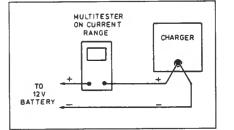
Fig. 6. Checking the current flow into a battery.
