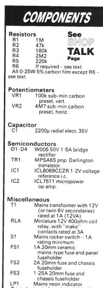
Printed circuit board available from the *EPE PCB Service*, code 934; 8pin d.i.l. socket; aluminum box, size 150mm x 100mm x 60mm minimum; crocodile clips (or spade-type connectors) (2 off); solder tags; 12V bulb, lampholder and crocodile clips for testing – see text; sheet aluminium for p.c.b. mounting; small fixings; strainrelief bush; rubber grommet; stand-off insulators (3 off); multistrand connecting wire; solder etc.
