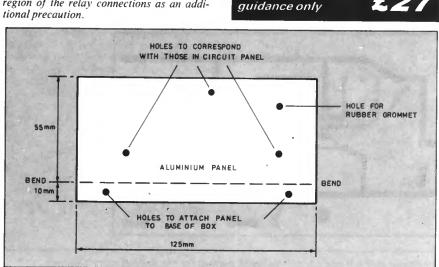
Fig. 3. Shaping the aluminium panel to which the p.c.b. is mounted.
