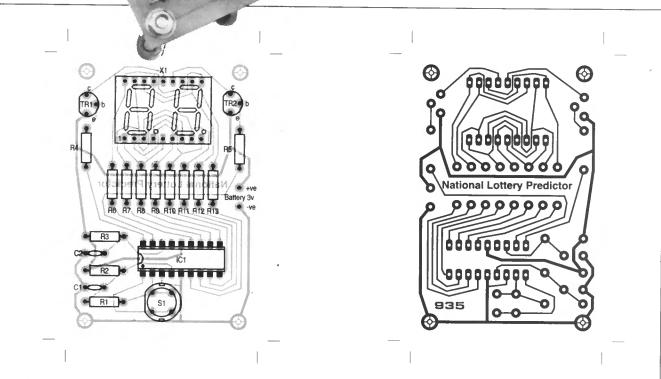
Fig. 5. Printed circuit board component layout and full size copper foil master pattern for the National Lottery Predictor.
