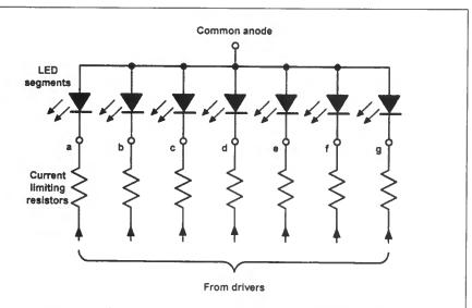
Fig. 7.29 Typical arrangement for a common-anode seven-segment display.
