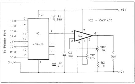
Fig. 1. The PC printer port D/A converter circuit diagram.
