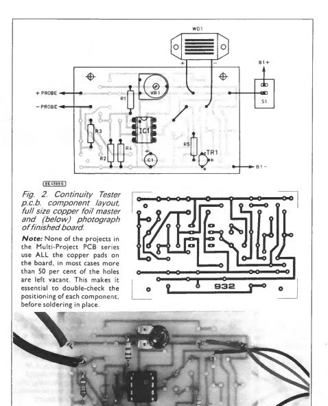
prods connected together the buzzer should not operate.
