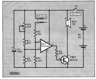
The two inputs of IC1 are fed from separate potential dividers. Preset VR1 and resistors R1 and R2 provide a reference potential to the inverting input, pin 2, and this voltage can be adjusted by means of VR1. Resistors R3 and R4 form the potential divider at the non-inverting input, pin 3, and these provide an output voltage equal to half the supply potential.
