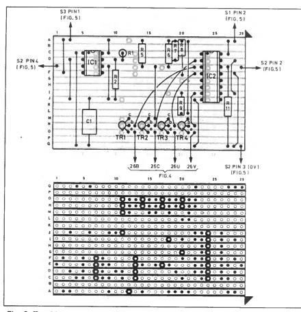
Fig. 2. Topside component layout and underside stripboard track cuts and solder joints for the Clock Generator and Large Number counter board.
