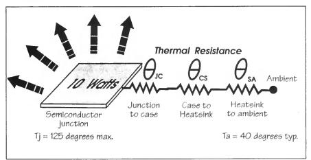
Fig. 2. Thermal resistance present in a heatsink system.
