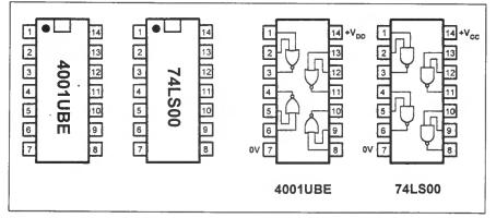
Fig. 7.18 Example of markings on digital integrated circuits.
