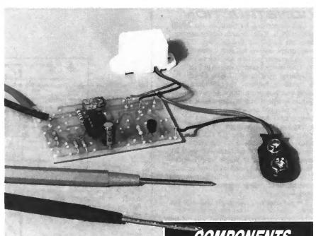
voltage. Under standby conditions there is an extremely high resistance across the test probes, giving zero volts at IC1's non-inverting input. The inverting input is therefore at the higher voltage, and the output of IC1 is low. This results in transistor TR1 being cut off, and the buzzer (WD1) is switched off.
