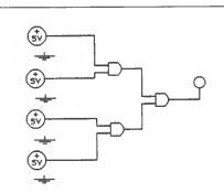
Fig. 7.21 Multiple-input AND gate (Assignment 7.2).
