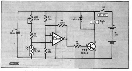
Fig. 1. Circuit diagram for the Light Activated Switch.
