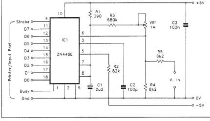
Fig. 2. Circuit diagram for the printer port A/D convertor.
