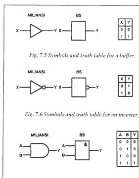
Fig. 7.7 Symbols and truth table for a two-input AND gate.
