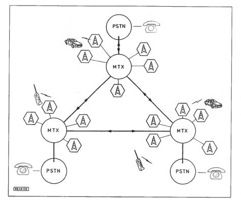
Flg. 4. How mobile telephone exchanges (MTX) are interlinked to form a comprehensive grid.
