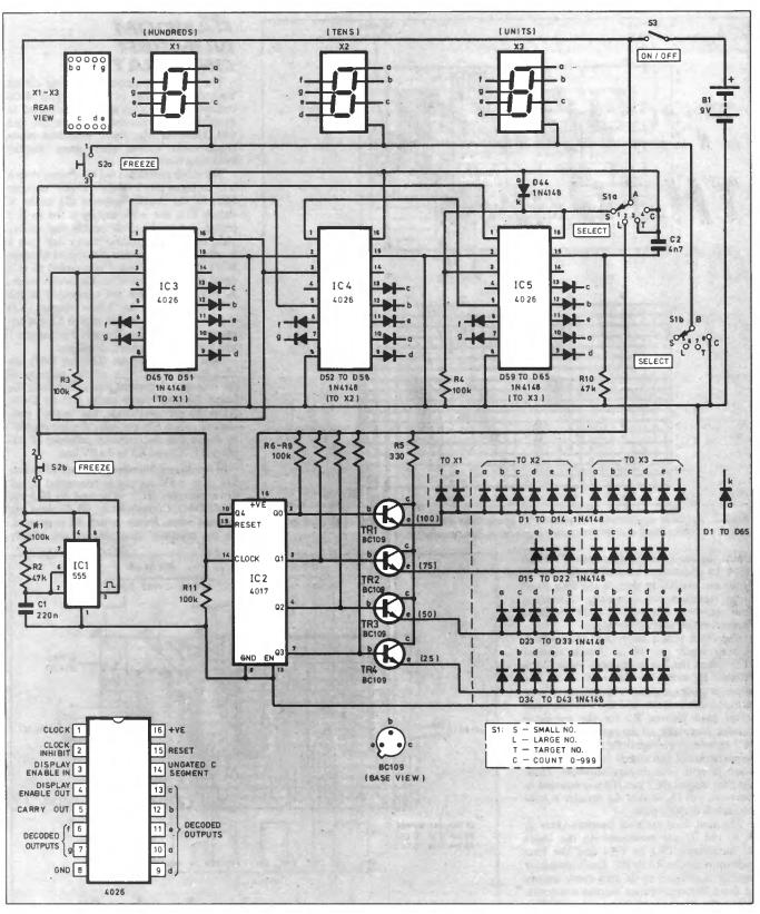
Fig. 1. Circuit diagram for the Counterspin games unit.
