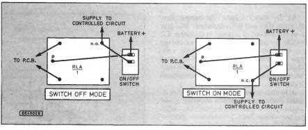
Fig. 3. Two methods of wiring the relay to the existing control equipment on/off switch.
