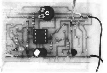
Layout of components on the printed circuit board.
