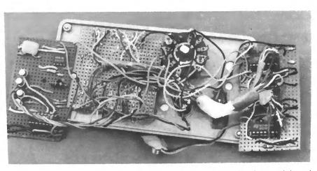
Photograph showing the interconnecting cabling between the three stripboard assemblies and the switches.
