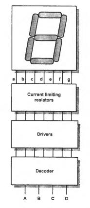
Fig. 7.30 Decoded seven-segment display showing binary-coded decimal (BCD) input (labelled A to D).
