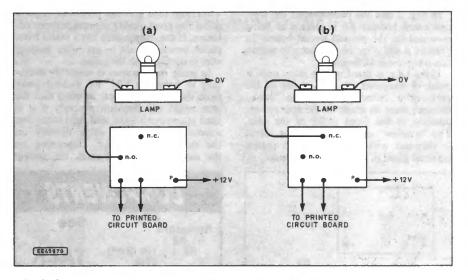
Fig. 3. Contact connection details when using the specified 10A relay. (a) to switch the lamp ON when the light threshold level is exceeded, and (b) to switch if OFF when the threshold level is exceeded.
