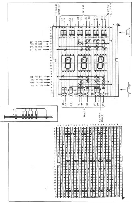
Fig. 4. Topside component layout and underside stripboard track cuts and solder joints for the Display/Matrix board. The insert shows an example of how the vertically mounted diodes should be connected.
