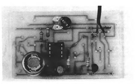
The completed circuit board with the l.d.r. (light sensitive resistor) mounted directly on the p.c.b.
