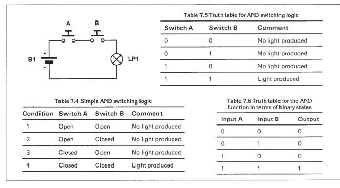
Fig. 7.2 AND switching logic with truth tables.
