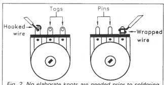
Fig. 2. No elaborate knots are needed prior to soldering wires in place.
