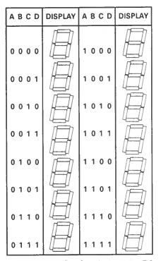
Fig. 7.34 Results for Assignment 7.3 (decoded display).
