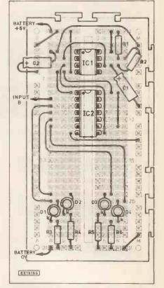
Fig. 28.2. Circuit diagram for investigating a shift register.
