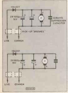
Fig. 3. Circuit diagram for type "A" (top) and type "B" cars.
