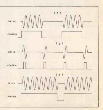
has to be emphasised that this method of power control is not suitable for all types of equipment. It is well suited to the control of heating elements, but does not work properly with lamps. With the latter its effect is to flash the lamp on and off at a rate of a few Hertz, although I suppose the unit does have possible application as an interference-free lamp flasher.
