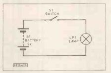
Fig. 1.8. Adding a switch in circuit.
