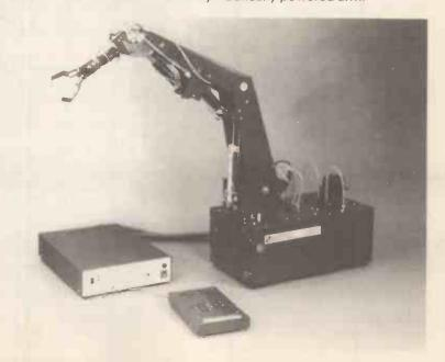
directions, lift 2kg, vacuum or twofingered pneumatic gripper. Software for IBM can network with up to seven other Cybernetic machines and work cell. £3,870 plus VAT.
