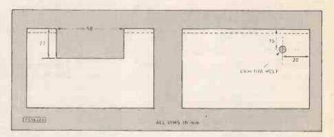
Fig. 4. Dimensions, cutting and drilling details for the ends of the case. Note that the slider cutout is the opposite end to the p.c.b.
