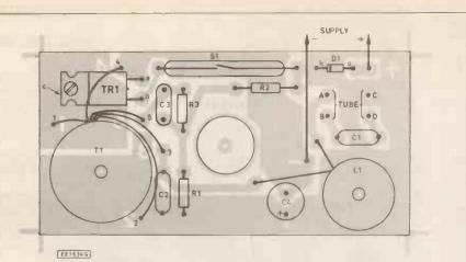
Fig. 6. Printed circuit board component layout. The centre of the board is cut out to take the u.v. tube.
