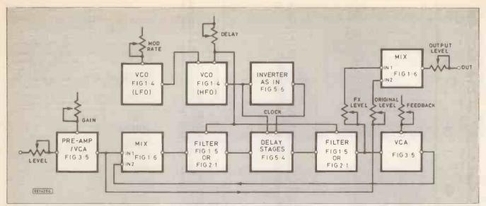
Fig. 5.7. Block diagram for a multipurpose unit for producing such effects as: reverb, phasing, flanging, double tracking and vibrato.
