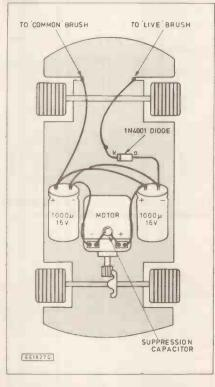
Fig. 6. Modification details and wiring for type "B" car.
