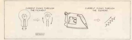
Fig. 1.5. Current must flow through the "component" in order for it to perform its function.
