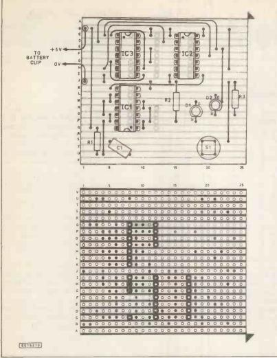
Fig. 28.8. Stripboard component layout and underside view, showing breaks in the copper strips, for the Pseudo-random Head or Tails? Make sure that all link wires are correctly positioned.
