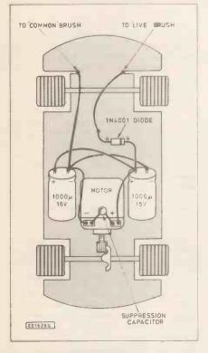
Fig. 5. Modification details and wiring for type "A" car.
