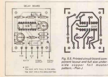
may be used in conjunction with many of the circuits already described, and several may be chained together to extend the delay time.
