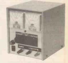
A superb design giving 0-25V and 0-2.5A. Twin par meters indicate Voltage and Current. Voltage is va able from zero to 25V. Current-Limit control allows Constant Current char
