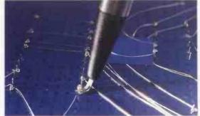
4. Changes are simple too – the unwrap tool is used to remove the connections so the component can be re-used.
