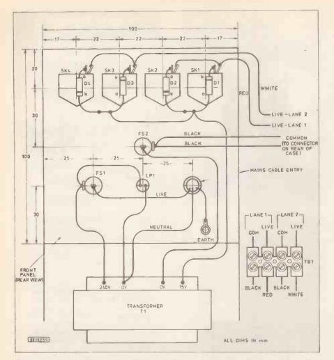
Fig. 4. Front panel layout, drilling details and interwiring for the main power supply unit. The track connecting terminal block TB1 is mounted on the outside of the rear panel.
