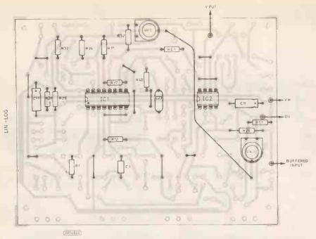
Fig. 5.3. Printed circuit board component layout for the Lin-to-Log Converter-—Plan 1. The full size printed circuit copper foil master pattern appeared in Part One (June '88), Fig. 1.1.
