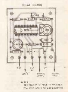
Fig. 5.8. Component layout for a Simple Reverb Controller combining two boards—Plan J and Plan K.
