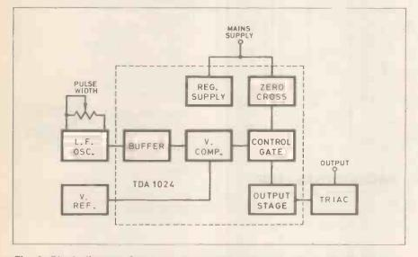
Fig. 3. Block diagram for the controller based around the TDA1024 triac i.c., incorporating zero crossing detection circuit.
