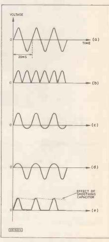
Fig. 1. Example waveforms showing various stages of operation. (a) 50Hz a.c. voltage from transformer; (b) full-wave rectification into pulsating d.c.; (c) and (d) independent control of positive and negative half cycles from transformer; (e) effect of car reservoir smoothing capacitor on the waveform.
