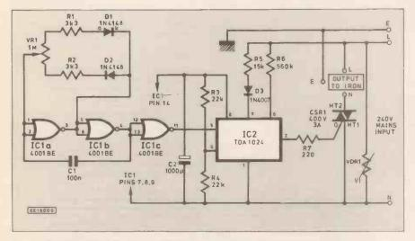
Fig. 4. Full circuit diagram for the Soldering Iron Temperature Controller.
