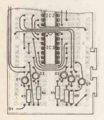
this is a *serial- in/parallel-out* register, or SIPO for short.
