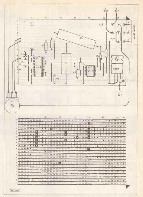
Fig. 5. Stripboard component layout, interwiring and details of breaks required in underside copper strips. (below) The completed board showing the high wattage resistor R5.
