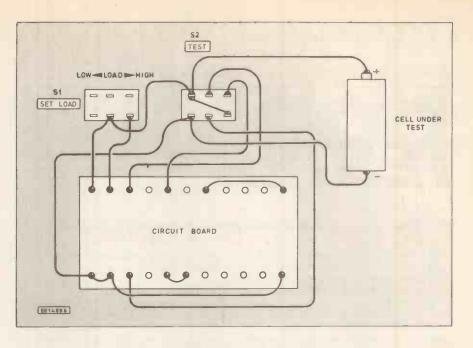
Fig. 3. Interwiring for the Battery Tester
