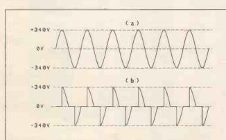
Fig. 1. Phase type a.c. power controllers cut out part of each half cycle to give reduced output power. (a) sinewave, (b) half power operation.
