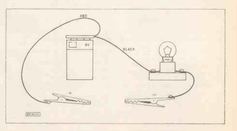
Fig. 1.6. Demonstration assembly to show current flow.
