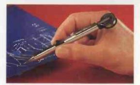
1. The special tinned copper wire – rated at 1 A – feeds smoothly through the pen from the reel fixed to its top, constructing the connection.
