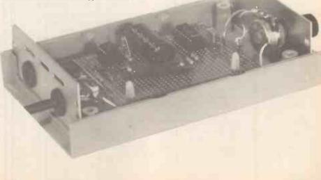
Therefore, once a high ouput level has been received from the comparator, the control gate will not provide a high output level until a zero cross-over of the mains signal has been detected.
