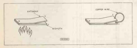
Fig. 1.4. Heat can be used to create electricity.
