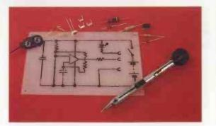
You can sketch your circuit directly on to the board and use it as a wiring diagram.
