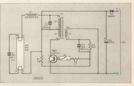
Fig. 1. Complete circuit diagram for the EPROM Eraser.
