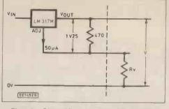
Fig. 2. Simplified regulated power supply arrangement. The value of  $\mathbf{R}_V$  can be found by referring to Table 2.
