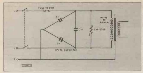
Fig. 4. Mains input suppression of earthed equipment.
