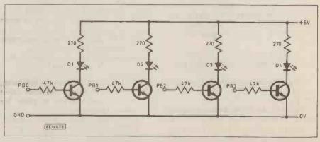
Fig. 9.2. Representative I.e.d. driver arrangement.
