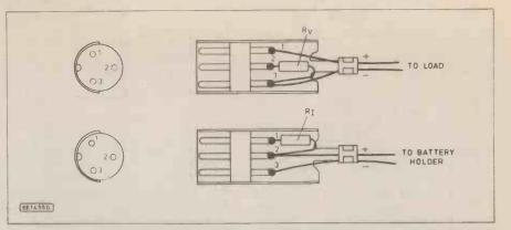
Fig. 5. Wiring to the DIN plugs for power supply and charger mode. It is suggested that the resistor leads are covered with insulating sleeving to avoid shorting to the other pins.
