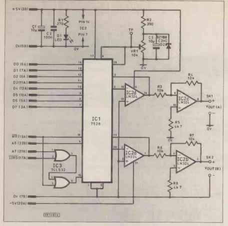
Fig. 4. Complete circuit of the Spectrum Dual DAC.
