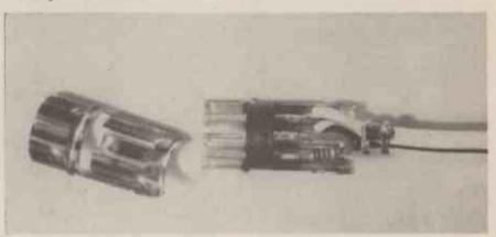
soldered to pins on the circuit board. If a chassis type socket is used a suitable hole should be drilled in the case and short wires soldered from the circuit board pins to the socket tags. As the components are such a tight fit inside the case it might be best if constructors kept to the "wander" type DIN socket method.
