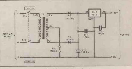
Fig. 4. Power supply circuit.
