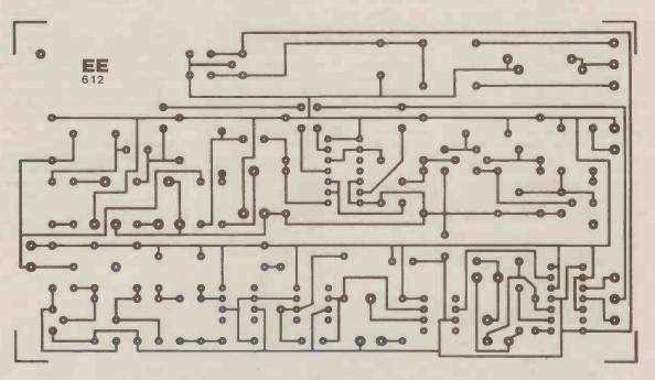
Fig. 5. P.c.b. layout for the Video Wiper.
