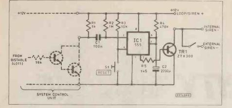
Fig. 2.2. Time-Limited alarm circuit.
