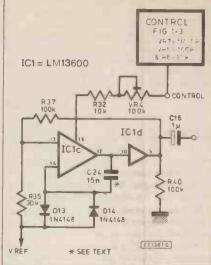
Fig. 2.6. Circuit diagram for a simple voltage controlled oscillator (VCO). The output waveform is shown in photograph 6.
