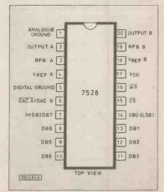
Fig. 5. Pin connections for the 7528 Dual DAC.
