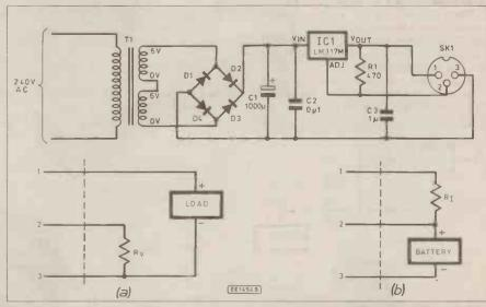
Fig. 1. Full circuit diagram for the Universal Charger/Power Supply. The two small diagrams are for (a) power supply mode and (b) charger mode.
