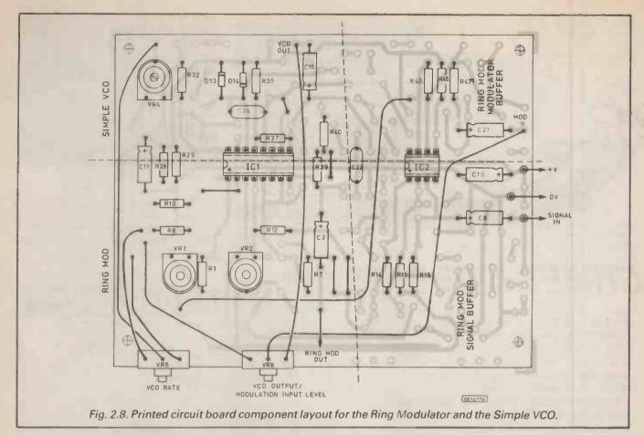
In essence two signals are brought together. They are not combined as happens in a mixer, but instead they intermodulate. Normally the speech or music signal goes to one input and an oscillator signal to the other.
