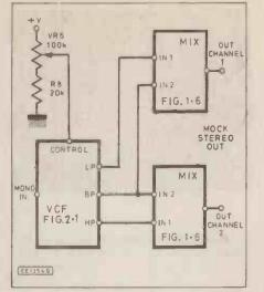
Fig. 2.4. Arrangement for producing mock stereo. The bass frequencies will be heard one side and high frequencies the other.
