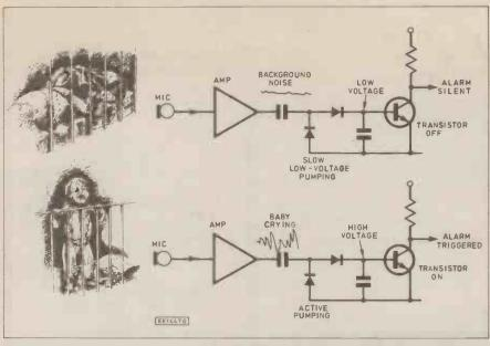
Fig. 25.5. One suggested application for the diode pump is as a Baby Alarm. With small background noise, amplifier output is low (alarm silent). When baby cries, output levels shoot up, switching transistor on and triggering alarm circuit.
