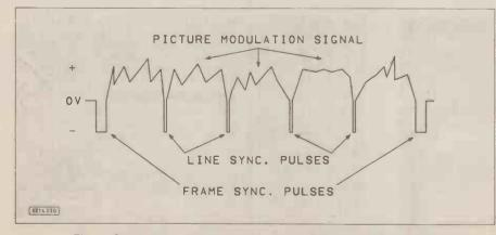
Fig. 1. Simplified representation of a composite video signal.
