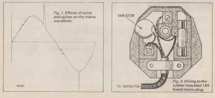
soon as a transient happens along, the device switches to a low resistance state, dissipates the transient's energy as heat, and then reverts to its virtually non-conductive state.
