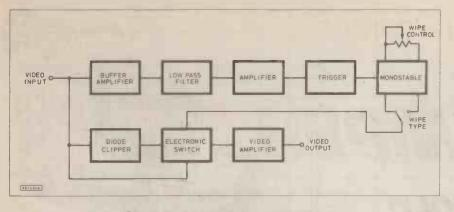
Fig. 2. The video wiper block diagram.
