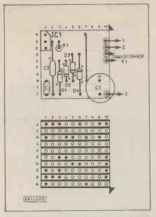
Fig. 4. Component layout and details of wiring to the mains transformer secondary winding and to the DIN socket.
