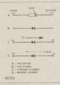
Fig. 25.1. The semiconductor diode.
