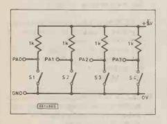
Fig. 9.1. Representative switch input arrangement.
