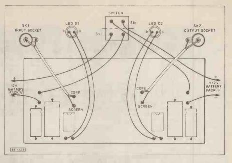
Fig. 4. Interwiring from the circuit board to the switch, l.e.d.s and sockets mounted on one side of the plastic case.
