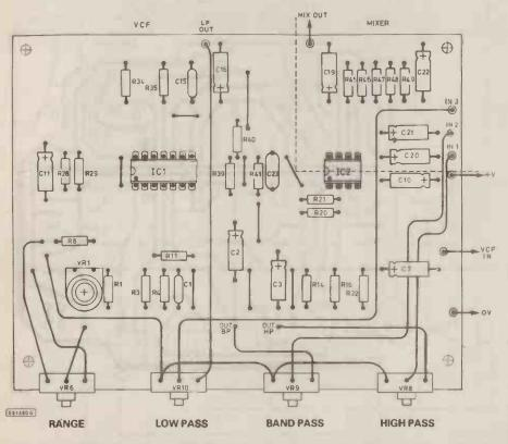
Fig. 2.2. Printed circuit board component layout for the VCF and Mixer. A full size copper foil master pattern was given in Part One, last month.
