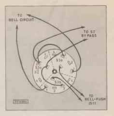
Fig. 2.6. Wiring of the exit door switch.
