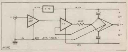
Fig. 3. Audio amplifier with split (dual, centre-tapped) supply for the power amplifier (P.A.) part and a reduced-voltage single ended supply for the low-level stages. Note the common ("earth") connections, where separate lines are provided for PA and preamp, joined only at the tags of the reservoir capacitors in the power supply.
