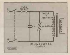
Fig. 5. Mains input suppression of NON-earthed equipment.
