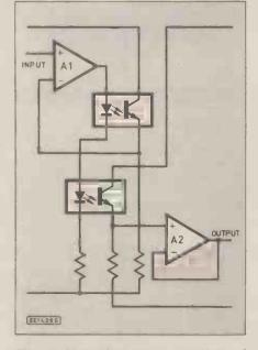
Fig. 1. Simplified representation of the opto-link circuit stage.
