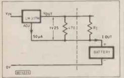
Fig. 3. Simplified arrangement for charger operation. The value of the charging resistor  $\mathbf{R}_{I}$  can be found by referring to Table 3.
