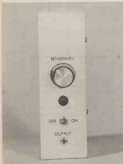
(Left): Receiver front panel layout. (Above): The completed transmitter and receiver. The mounting adaptor can be seen on the side of the transmitter.
