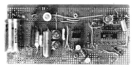
The completed generator circuit board showing positioning of components.
