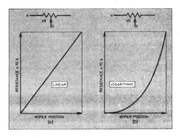
Fig. 2.5 (a) A linear potentiometer has a linear relationship between the wiper position and resistance whilst (b) a logarithmic potentiometer produces a non-linear graph.
