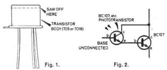
Take a transistor in a TO5 or TO18 can, such as a BC107, and, using a fine razor saw carefully remove the top of the transistor, taking care not to squash the can (see Fig. 1). Carefully shake out any particles of metal which may have fallen inside the transistor.
