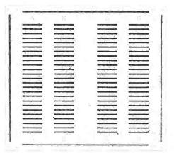
Fig. 2.9. Diagram of the Eurobreadboard indicating how individual sockets are permanently interconnected inside the board.
