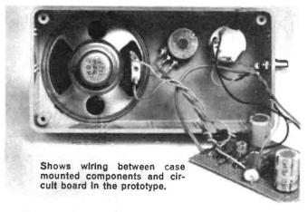
screened lead to connect to the input socket SKI was used in the prototype, but this is not essential.
