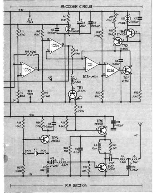
The code appearing on pins 9, 10 and 11 is changed by the counter in IC2 being clocked as already mentioned by the output of IC3b so as to present the next channels in sequence on to the output.
