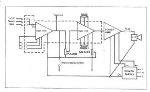
The HY5 pre-amp is compatible with all I.L.P. amplifiers and P.S.U.'s. It is contained within a single pack 50 x 40 x 15 mm. and provides multifunction equalisation for Magnetic/. Ceramic/Tuner/Mic and Aux (Tape) inputs, all with high overload margins, Active tone control circuits; 500 mV out. Distortion at 1KHz-0.01%. Special strips are provided for connecting external pots and switching systems as required. Two HY5's connect easily in stereo. With easy to follow instructions.
