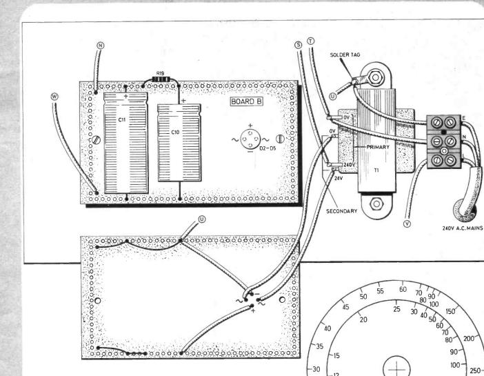
Fig. 4. Shows the power supply circuit board and transformer mounted on the internal face of the rear panel, and interwiring.
