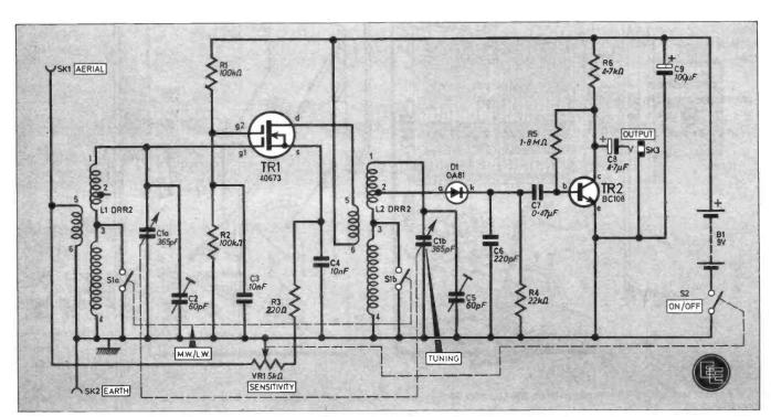
Fig. 1. The complete circuit diagram for the Medium and Long Wave Radio Tuner.
