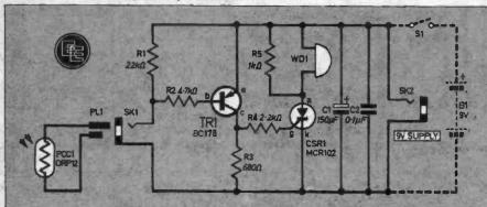
Fig. 1. The circuit diagram of the Opto Alarm. The dotted components replace SK2
