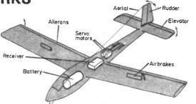
The information starts out as a voltage across a potentiometer connected to the control sticks. This voltage is their converted into a digital pulse whose width is proportional to the voltage. Several of these pulses are grouped together into a series pulse train, one for ead function to be controlled, and the whole train is repeated 50 times each second to enable changes in information to be quickly transferred to the model
