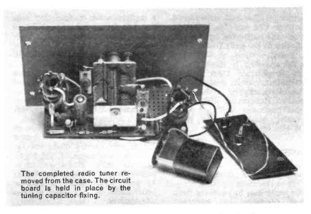
to lock against the capacitor and panel. This capacitor provides sufficient support for the board.
