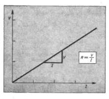
Fig. 2.1. Plotting current against voltage shows there to be a straight line (linear) relationship between the two. The slope of the graph gives the resistance.
