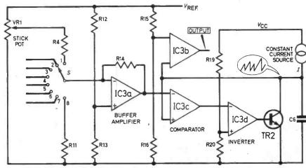
Fig. 1.2. Linear Ramp Encoder: basic circuit.
