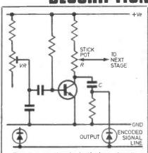
Fig. 1.1. A simple half-shot circuit. This works on a *CR* charging curve where the charging time is determined by the stick pot position. This circuit would be repeated for each channel, and require the setting up of seven pre-set pots.
