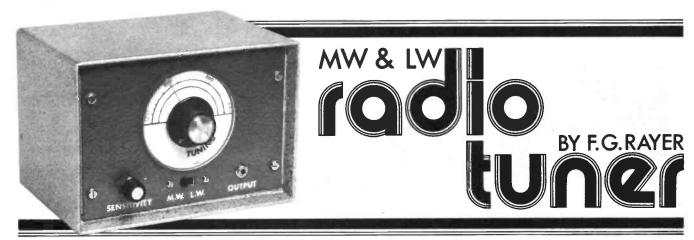
A TUNER to provide a.m. reception on medium and long wave bands increases the scope and entertainment value of an audio amplifier. This tuner has sufficient output for even insensitive amplifiers, while avoiding the relative complication of a superhet circuit. Coverage is approximately 1600 to 600kHz m.w., and 490 to 185kHz l.w., or 360 to 145kHz l.w.
