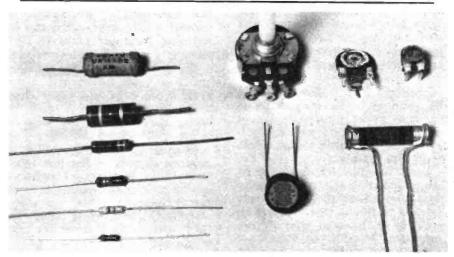
Typical resistors (left) a wire-wound 5 watt fixed resistor, and (below) carbon resistors ranging from 1 watt to 1/10th watt. (Top right) three variable resistors (potentiometer): standard control type and two miniature presets. (Bottom right) light dependent resistor and thermistor.
