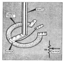
Fig. 2.4. The construction of a typical potentiometer.
