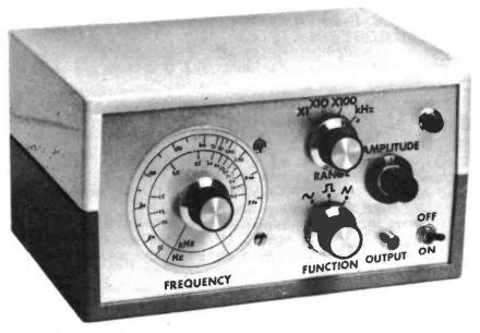
The sinewave signal has a minimum harmonic distortion factor of about 2 per cent when correctly adjusted but lower than this is not possible as the sinewave is obtained by electronic shaping within IC1 and not by pure generation.
