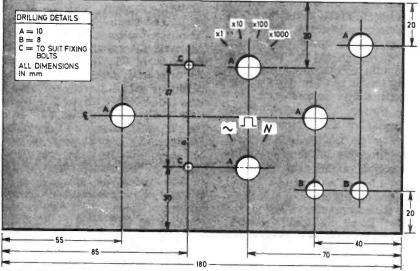
Fig. 2. Dimensions and drilling details for the front panel of the unit with some suggested panel markings.
