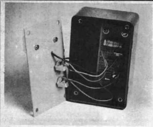
The completed Opto Alarm showing positioning of the circuit board and wiring to the jack sockets.
