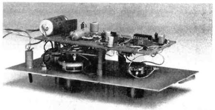
Mounting of the generator circuit board on the rear of the front panel.
