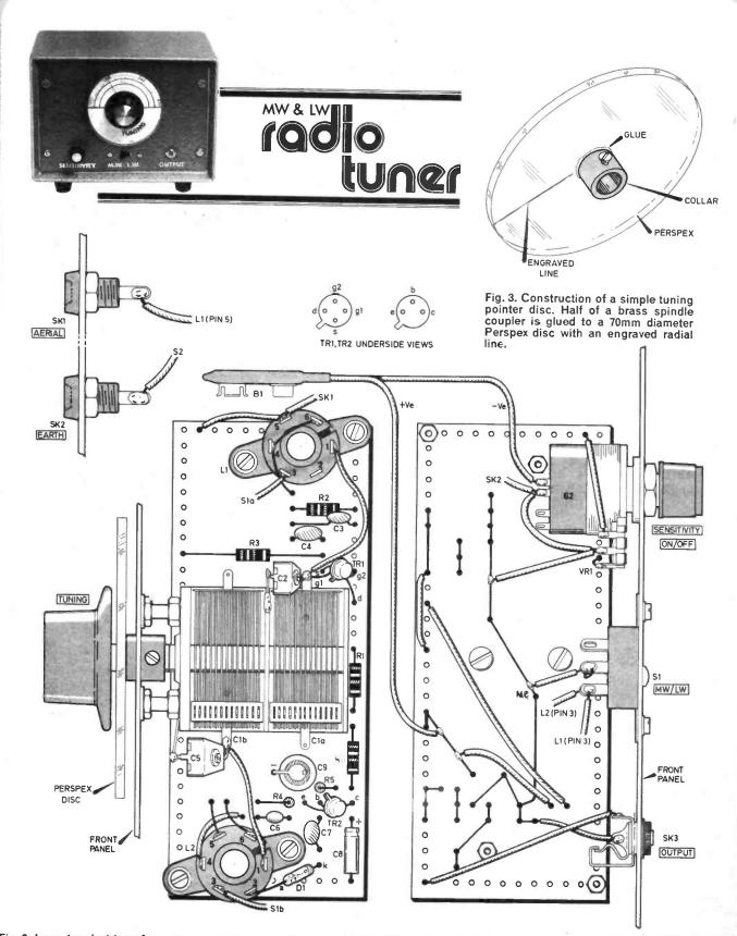
Fig. 2. Layout and wiring of components on the top and underside of the plain perforated circuit board and interwiring to panel mounted components.
