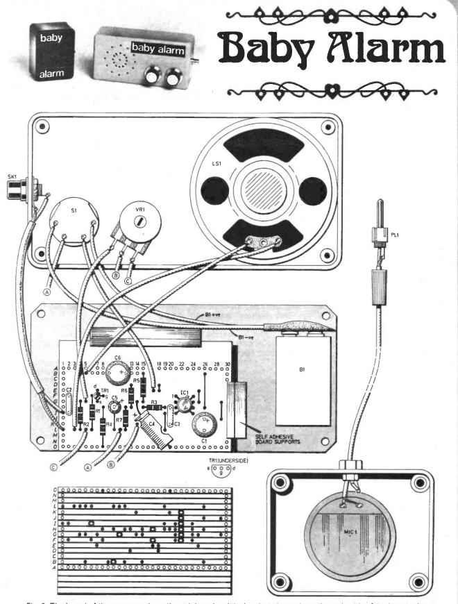
Fig. 2. The layout of the components on the stripboard and the breaks to be made on the underside of the board; also shown are components mounted to the case and position of battery and circuit board on base panel and full Interwiring. Bottom right shows mounting of microphone in case and connection to phono plug via screened cable.
