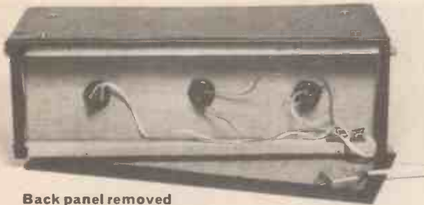
Back panel removed showing lampholder wiring.
