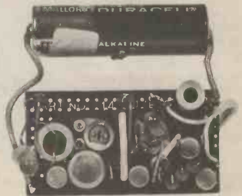
Photograph showing the completed circuit as built on a piece of stripboard.
